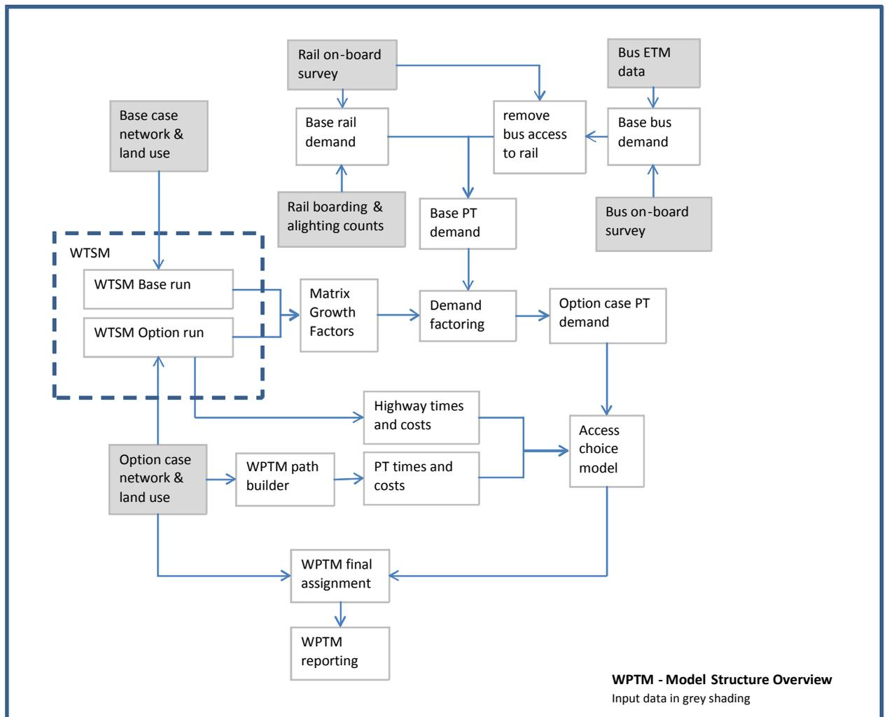
**Figure 2-1: WPTM Proposed Model Structure**
