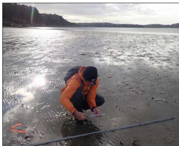
Measuring intertidal plates using a straight edge to average out any small-scale irregularities in surface topography
