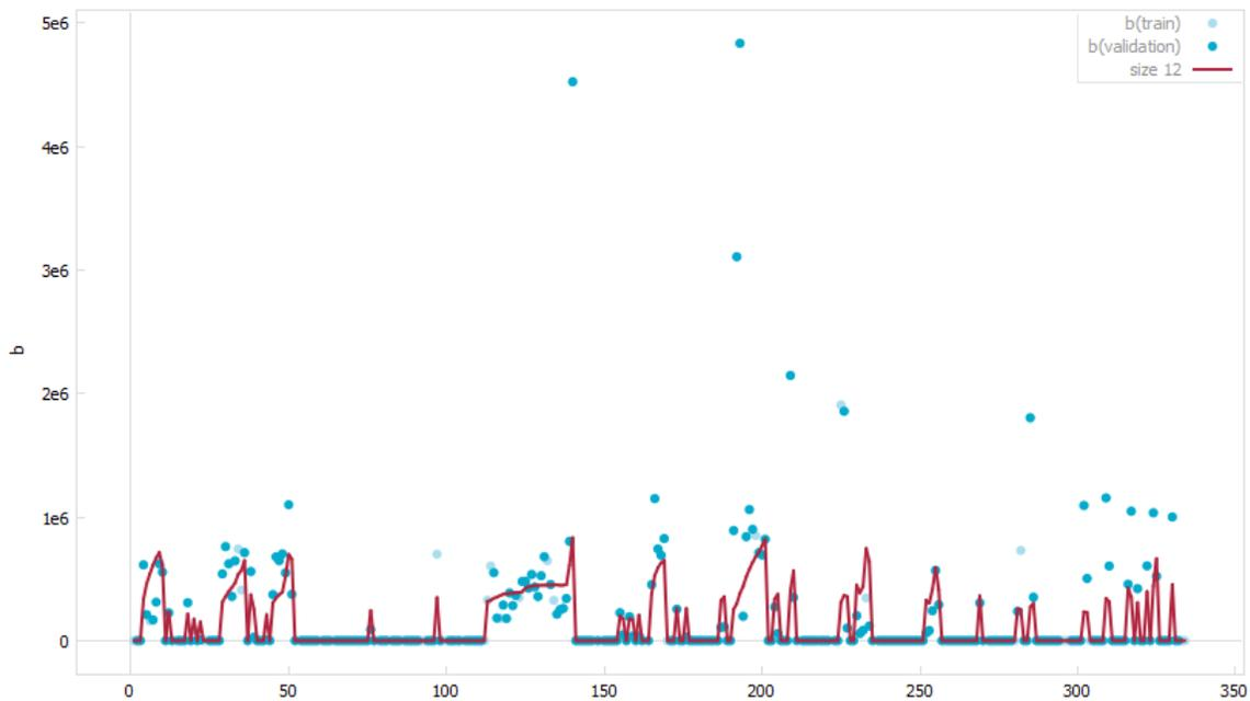
**Appendix Figure 1. Barrett inflow estimations (redline) compared to in situ measurements (blue dots).**
