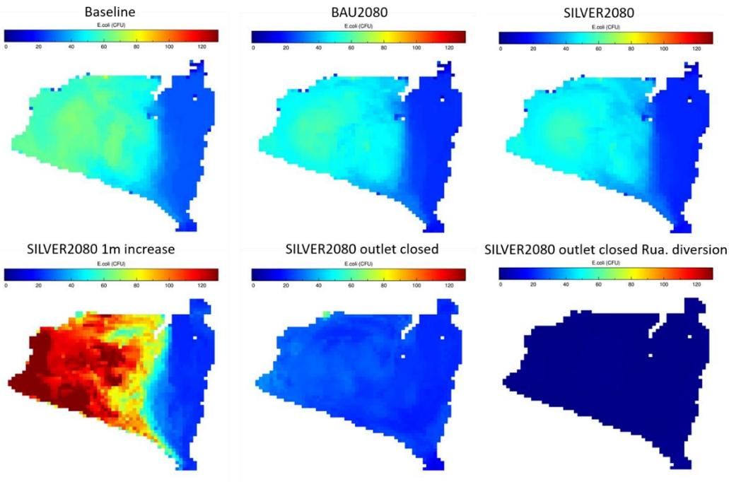
Figure 8. Median 3-D simulated *E.coli* concentration in Lake Onoke over a 91 day period beginning 1 Jan 2012 at 12pm. The scale runs from 0 to 130 CFU, with median 130 CFU being the swimmability boundary between excellent and intermittent. Note this is not
