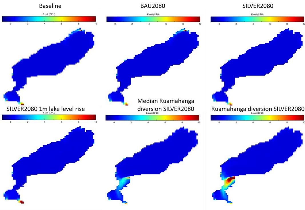
Figure 7. Median 3-D simulated *E.coli* concentration in Lake Wairarapa over a 91 day period beginning 1 Jan 2012 at 12pm. Note this is not calculated via Hazen methods, however all other NOF NPS related stats use Hazen. The scale runs from 0 to 10 CFU. Illustrative ONLY.
