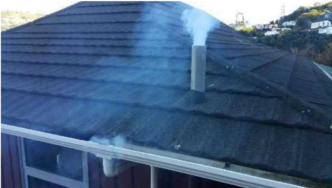
Figure 10. Smoke testing indicating presence of stormwater connections to the wastewater network. Image courtesy of Wellington Water ( https://www.wellingtonwater.co.nz/faqs/wastewater/smoke-testing/ )
