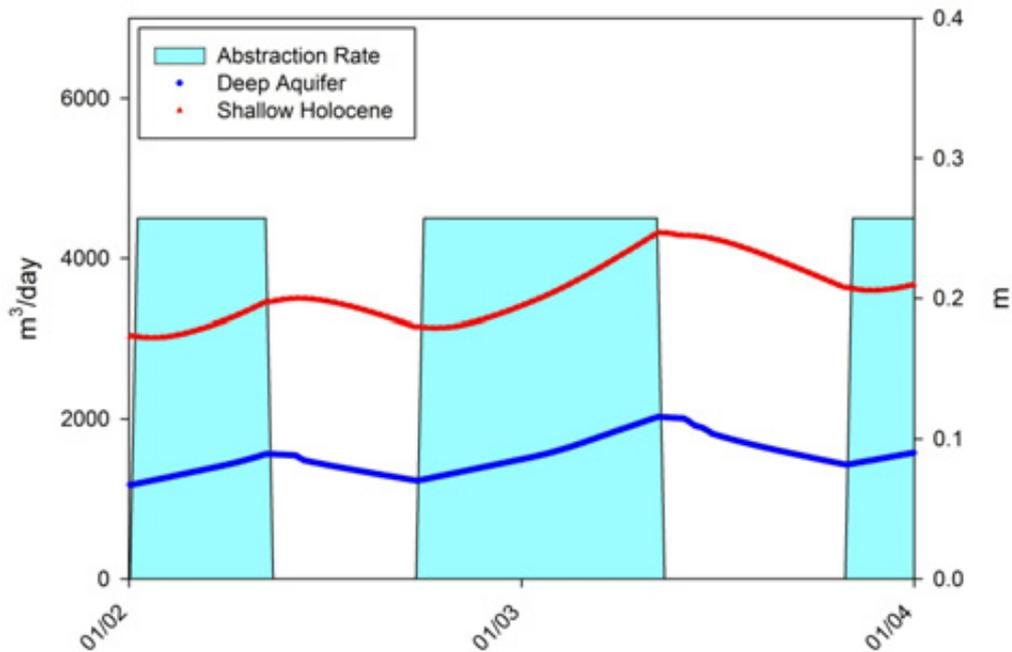
**Figure D12: Simulated drawdown associated with seasonal abstraction at 4,500 m<sup>3</sup>/day from the shallow Holocene aquifer and deep aquifer respectively over the 2002/03 period**
