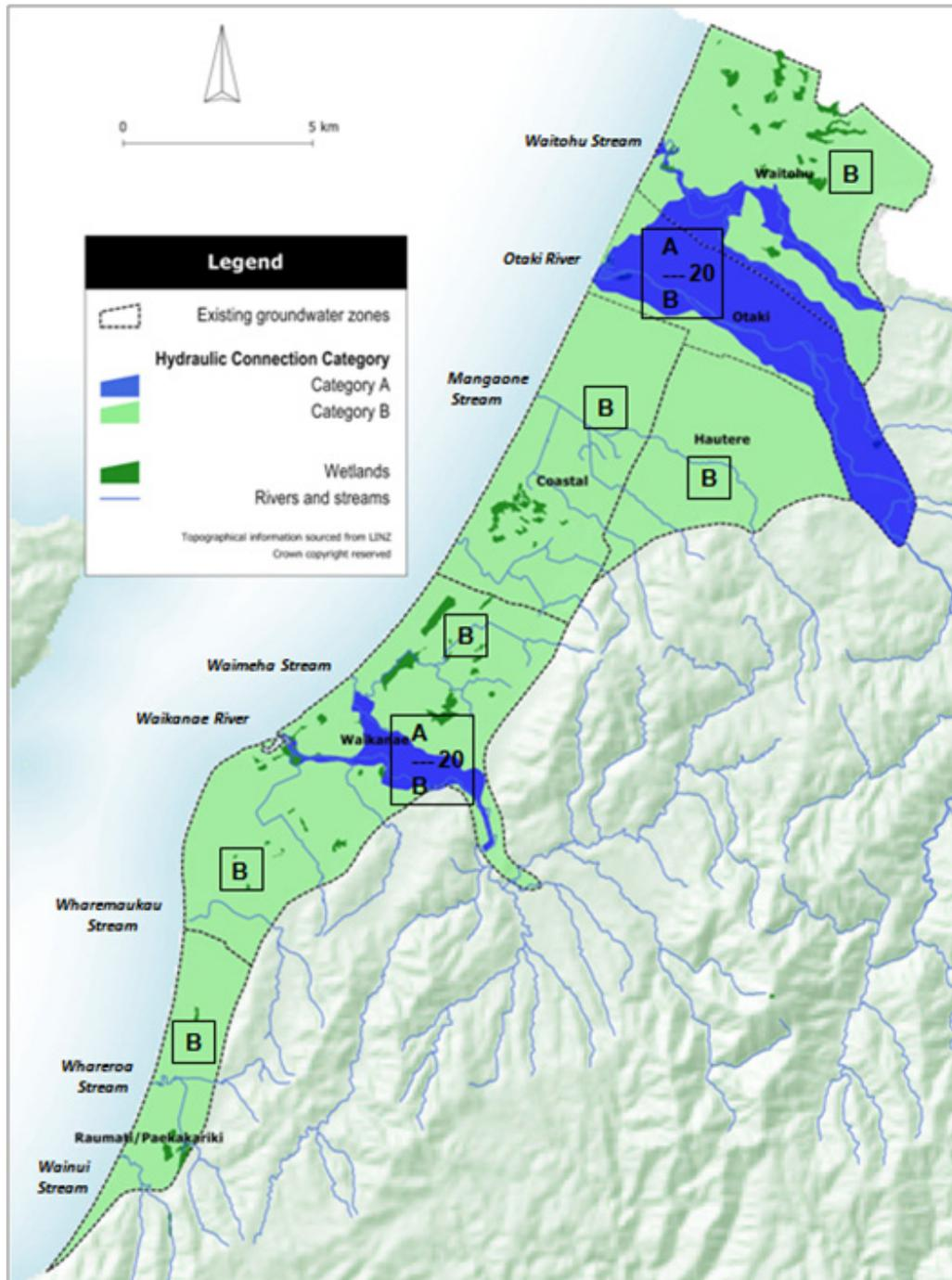
Figure 3.3: Spatial and depth distribution of proposed hydraulic connectivity zones for the Kapiti Coast
