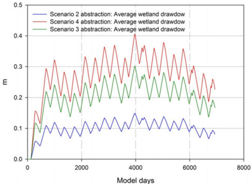
**Figure B9: Scenarios 2 to 4 – Wetland drawdown averaged over the six wetlands in the Te Hapua wetland complex. Wetland drawdown when wells are abstracting from all aquifers at 7,500 m<sup>3</sup>/day (Scenario 2), 15,000 m<sup>3</sup>/day (Scenario 3) and 20,000 m<sup>3</sup>/day (Scenario 4).**
