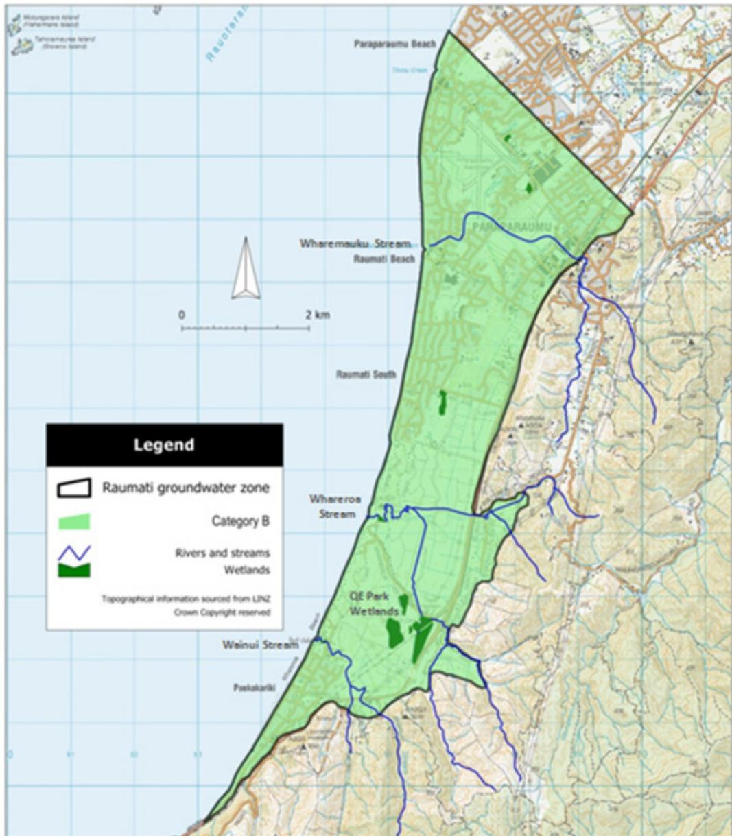
**Figure 4.6: Map of the proposed hydraulic connectivity zonation for the Raumati groundwater zone showing the location of significant surface water features**
