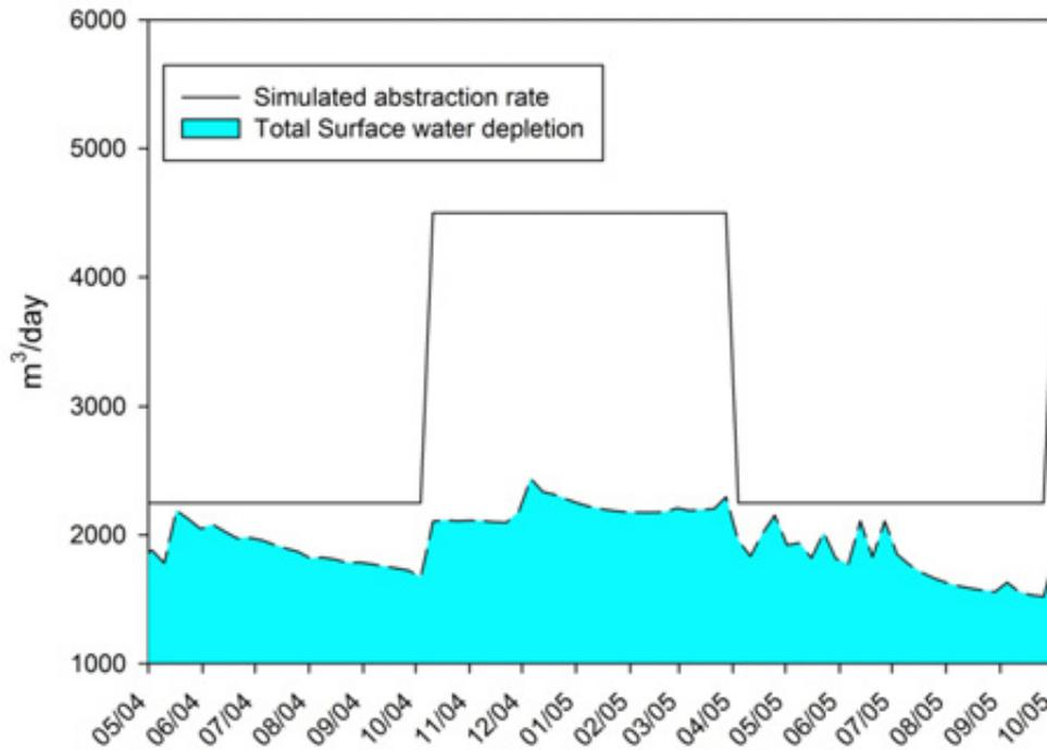
**Figure D14: Scenario 4 results – simulated cumulative stream depletion resulting from continuous abstraction (4,500 m<sup>3</sup>/day summer, 2,250 m<sup>3</sup>/day winter) between May 2004 and October 2005**
