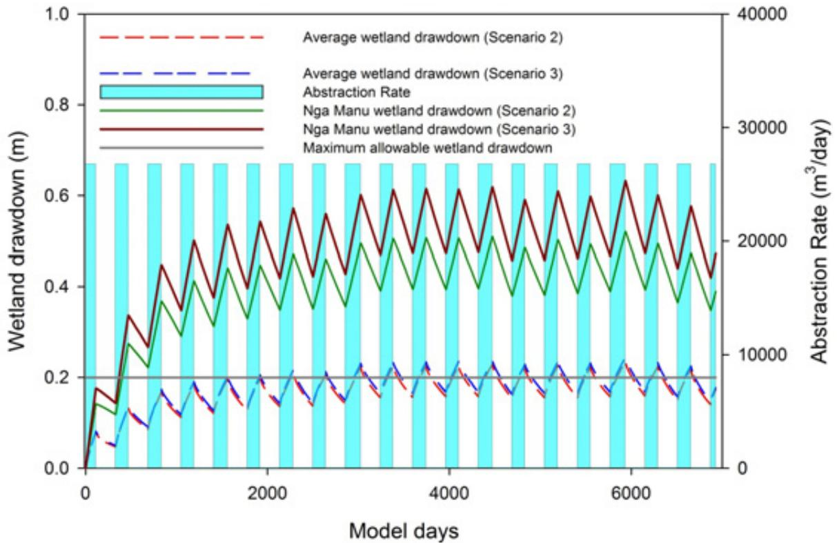
**Figure C13: Scenarios 2 and 3 – Simulated wetland drawdown for the Waikanae zone for 19 years of simulation at a seasonal pumping rate of 26,960 m<sup>3</sup>/day for scenarios 2 and 3. Plots show wetland drawdowns (average of 24 wetlands) and drawdown in the nationally significant Nga Manu wetland for the simulation period. The recommended maximum allowable abstraction effect on wetlands is a drawdown of 0.20m.**
