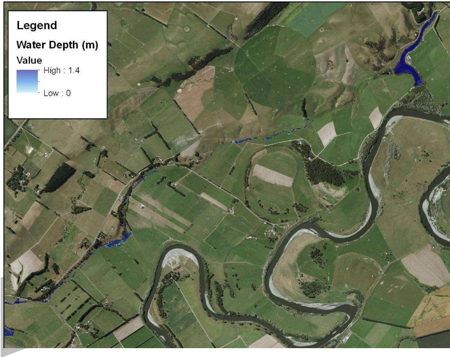
Figure 5-4 – Flood extent with upgraded conditions (Run 5), upstream of Pahautea Road
