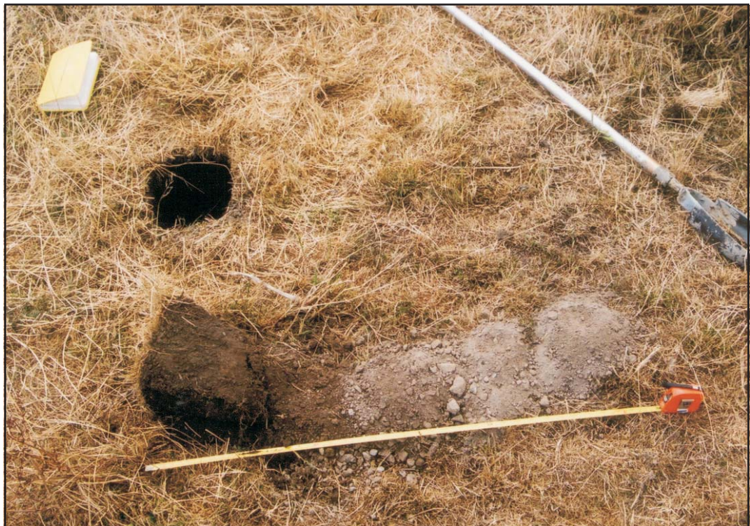
Figure 3. a) The fault scarp of the Mokonui Fault at the Viewfield site prior to trenching (NZMS 260 T26/320312). Four auger holes were drilled across the scarp to assess the subsurface stratigraphy. The total scarp height here is c. 3.2 metres. Water pumphouse occurs in the midground and farmhouse in the background. b) Auger hole and sediments retrieved adjacent to the Viewfield site. Gravels underlie c. 80 cm of fine-grained cover deposits.
