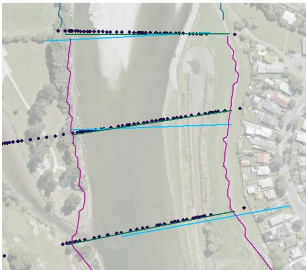
Figure 2.1: Cross sections 170-190 – 1998 bed with 2013 LiDAR bank levels
