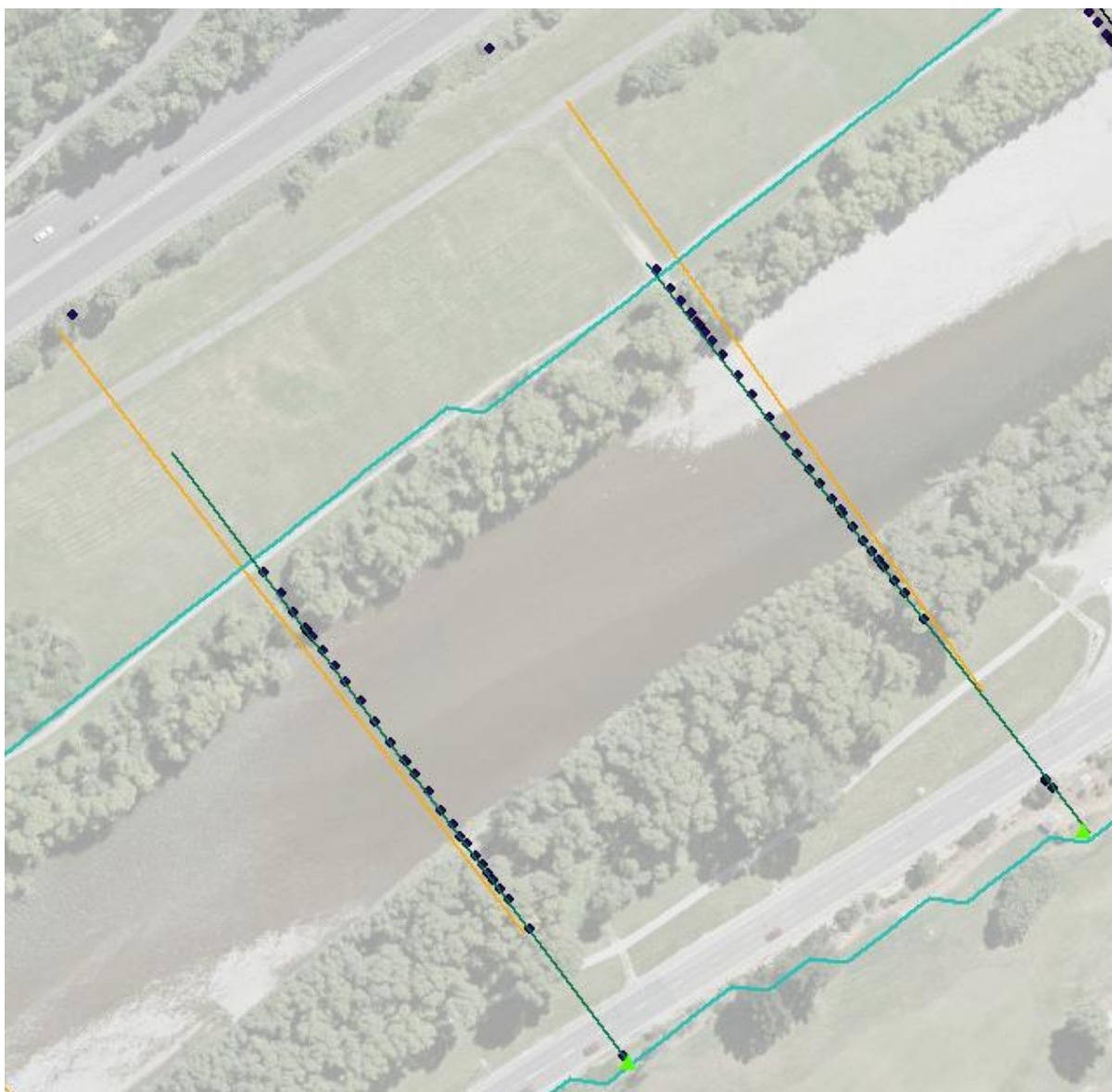
Figure 2.3: Cross-sections with only one bank level matched from the survey data.
