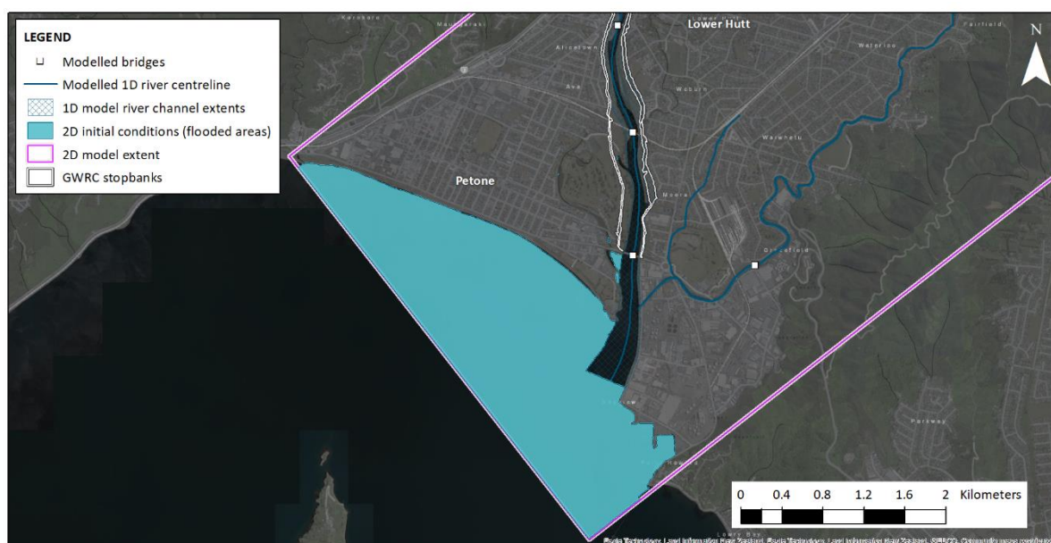
Figure 3.12: Spatial extent of 2D water level initial condition
