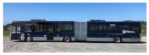
Figure 29: Example of an articulated bus
