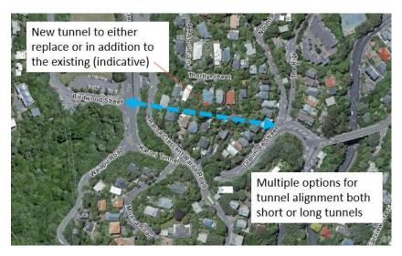
Figure 11: Indicative location for a new Karori road tunnel
