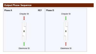
Figure 15: Phase sequence for Option 1q, full-time one-way operation of the tunnel
