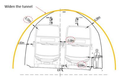
Figure 9: Option 1b - widening Karori Tunnel
