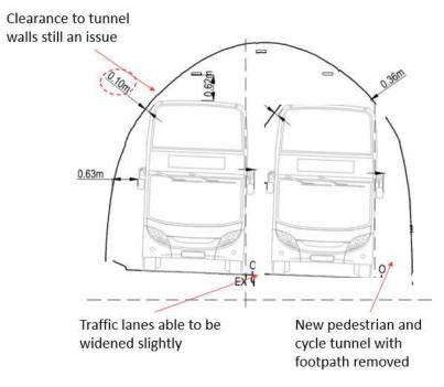
Figure 12: Option 1e - Karori Tunnel if footpath was removed
