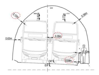
Figure 3: Karori Tunnel measurements (Source: Beca report)
