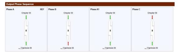
Figure 16: Phase sequence for Option 1h, partial one-way operation of the tunnel
