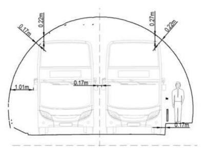
Figure 4: Seatoun Tunnel measurements (Source: Beca report)
