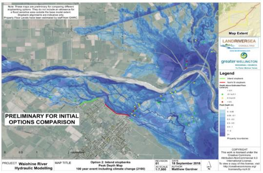
*Figure 3: Flood hazard map showing location of preferred stopbank option*
