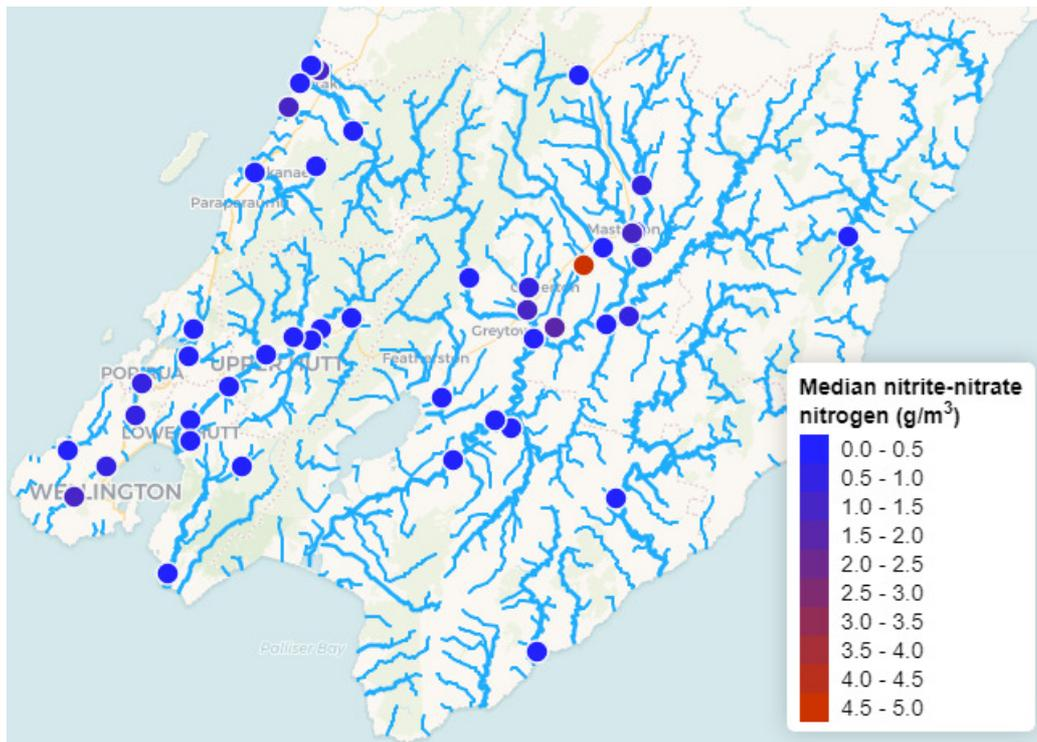
Figure 17: Nitrite-nitrate nitrogen ( $\text{g/m}^3$ ) results for the period 2019/20 to 2021/22
