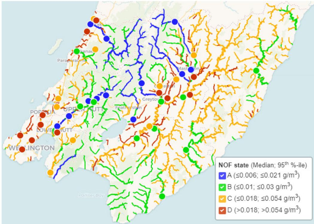
Figure 25: Dissolved reactive phosphorus (g/m<sup>3</sup>) NOF states for the period 2017/18 to 2021/22. See the methods [nutrients benchmarking section](#) for details.
