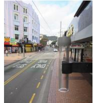
Street/Cuba Mall) and at Manners Street bus stop 5006 since August 2020. Passive diffusion tubes are a relatively inexpensive method that does not require a power source and provide useful information on long-term trends. The tubes are exchanged monthly using same method and sample exchange schedule as Waka Kotahi (NZTA). For further information see: <u>https://www.nzta.govt.nz/resources/air-quality-monitoring/</u>
