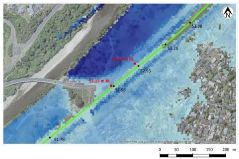
Figure 3 - Peak water levels in the 1 in 440 + CC or the 2,800 m3/s event
