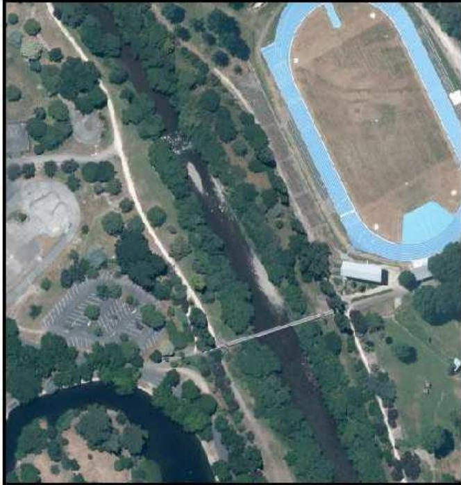
The flood risk from the Waipoua can be compounded by the backwater effects of flooding in the Ruamahanga River. Due to this the Waipoua was substantially modified and straightened in the 1930s and 1940s along with establishment of stopbanks.
