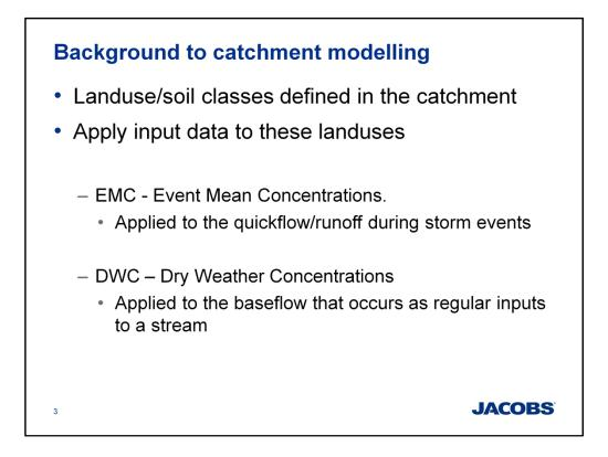
This slide summarises the approach undertaken to assign input concentrations in the model for E.coli to certain landuse types. There are 48 landuse/soil drainage combinations in the model, each with variations of E.coli EMC and DWC inputs.
