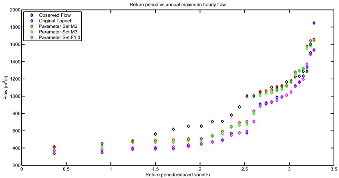
Figure 10. Observed versus modelled flood frequency data at Taita gorge versus the original TopNet calibration and three of the better performing re-calibrations (the M2 parameter set was the final one used).
