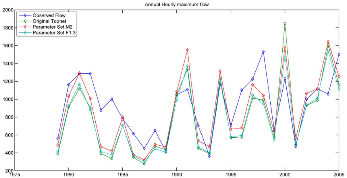
Figure 9. Observed flow at Taita gorge versus the original TopNet calibration and two of the better performing re-calibrations (the M2 parameter set was the final one used). Flow is given in cumecs.
