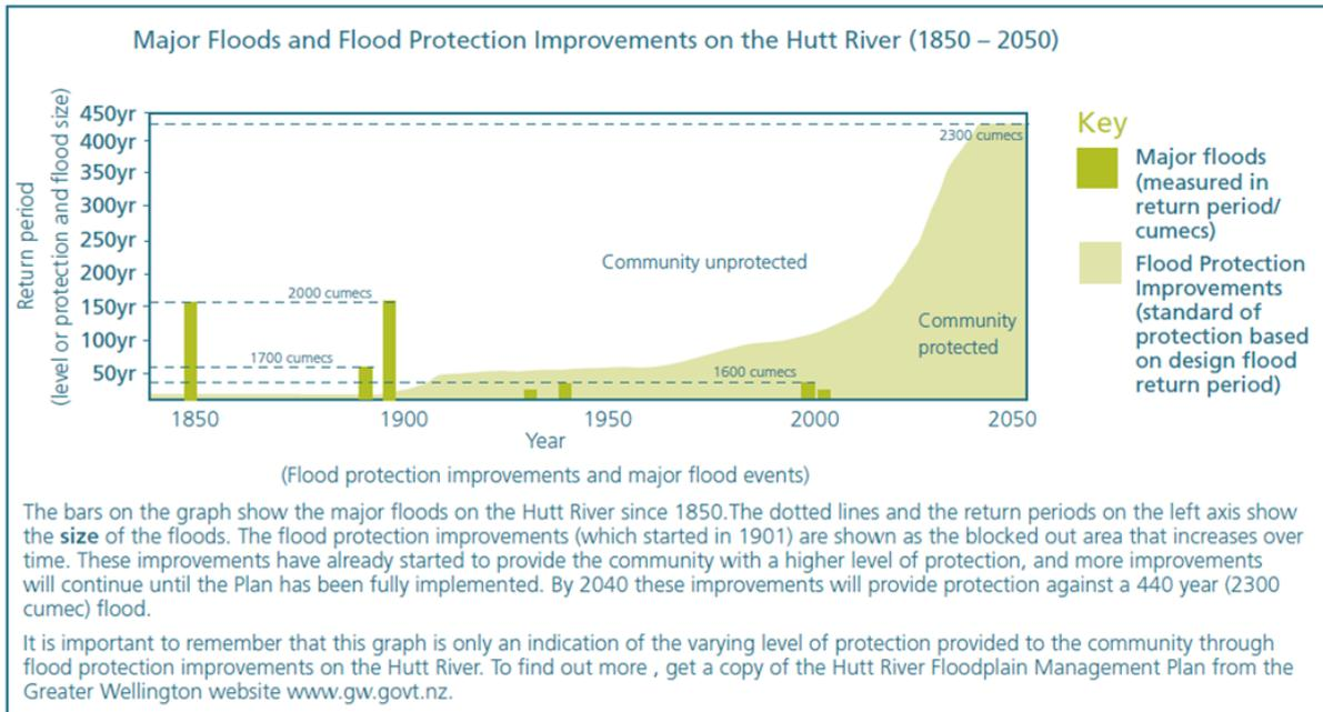
Figure 1. Flood protection improvements and community protection on the Hutt River Source: GWRC
