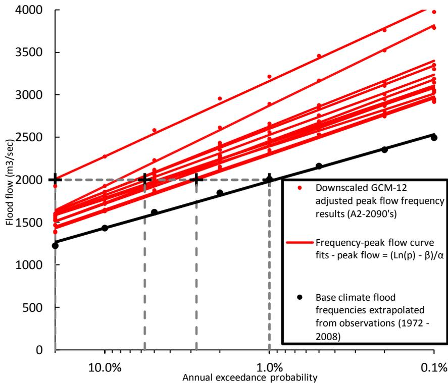
**Figure 8. Flood frequencies for the Hutt River at Taita Gorge under current (1972-2008) and modelled future climate (A2 emissions scenario, 2090s), corrected for the difference between modelled and observed flood volumes under current climate conditions (for details, see text).**
