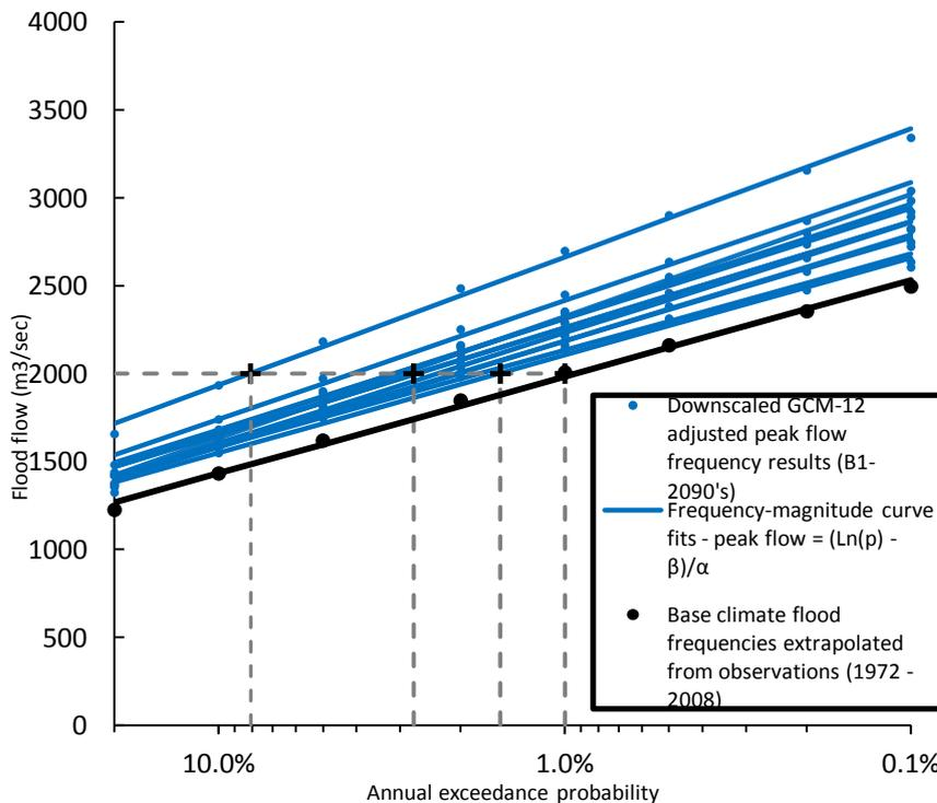
Figure 7. Flood frequencies for the Hutt River at Taita Gorge under current (1972-2008) and modelled future climate (B1 emissions scenario, 2090s), corrected for the difference between modelled and observed flood volumes under current climate conditions (for details, see text).
