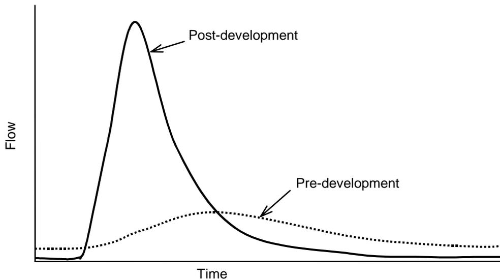
**Figure 1:** Schematic diagram of a typical storm hydrograph before and after a high degree of urbanisation showing the higher, sharper peak and reduced baseflow.
