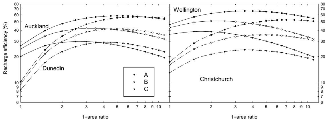
**Figure 10: Recharge efficiency for runoff areas in different cities and for three soil hydrologic groups. The calculations are based on rainfalls of  $1074 \text{ mm}$  for Auckland,  $1285 \text{ mm}$  for Wellington,  $646 \text{ mm}$  for Christchurch, and  $686 \text{ mm}$  for Dunedin. The area ratio is  $A_{id}/A_r$ , the impervious area leading to the runoff area divided by the runoff area.**
