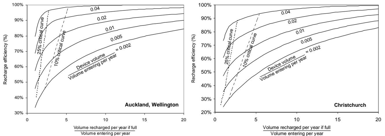
Figure 11: Recharge efficiency for various sizes of infiltration device.
