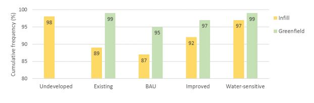
Figure 12. Cumulative frequency value corresponding to flow rate of 20 L/s across scenarios
