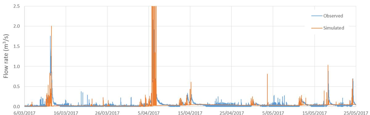
**Figure 4. Observed and simulated flow series used for model calibration**
