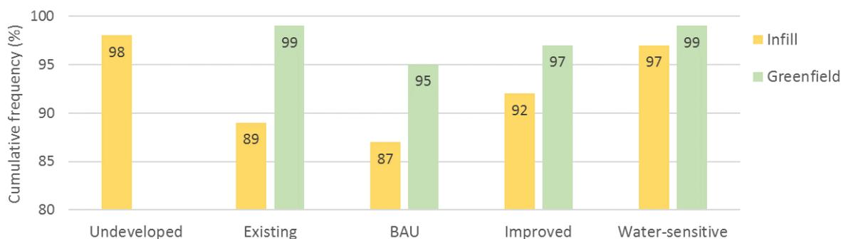
**Figure 12. Cumulative frequency value corresponding to flow rate of 20 L/s across scenarios**
