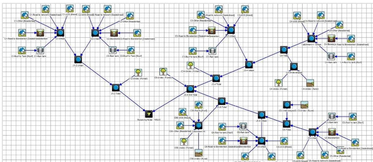
**Figure 5. MUSIC model showing source nodes, device nodes and receiving node**
