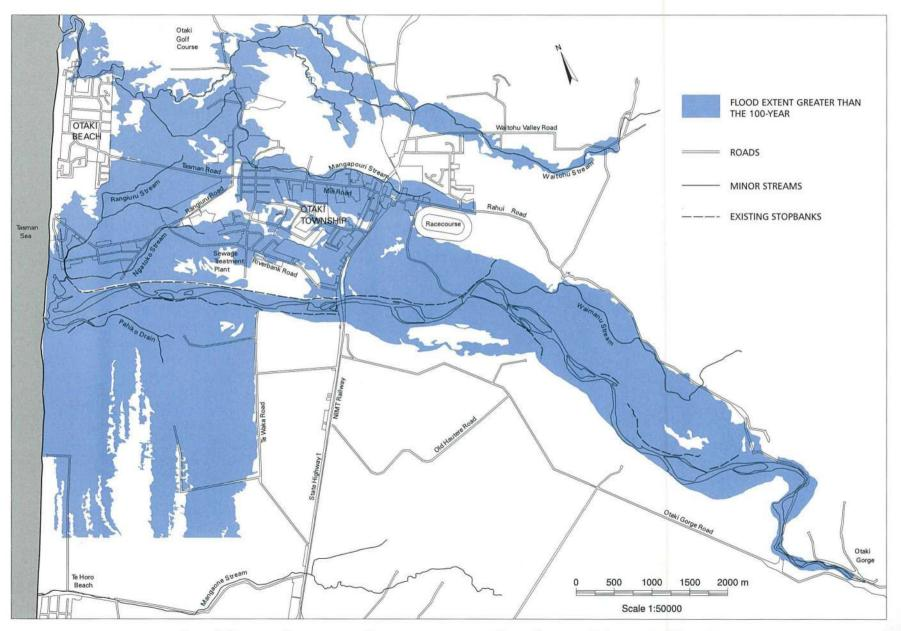
FIGURE 8: EXTENT OF FLOODING IN AN EVENT GREATER THAN THE DESIGN STANDARD (1.5 TIMES THE 100-YEAR)
