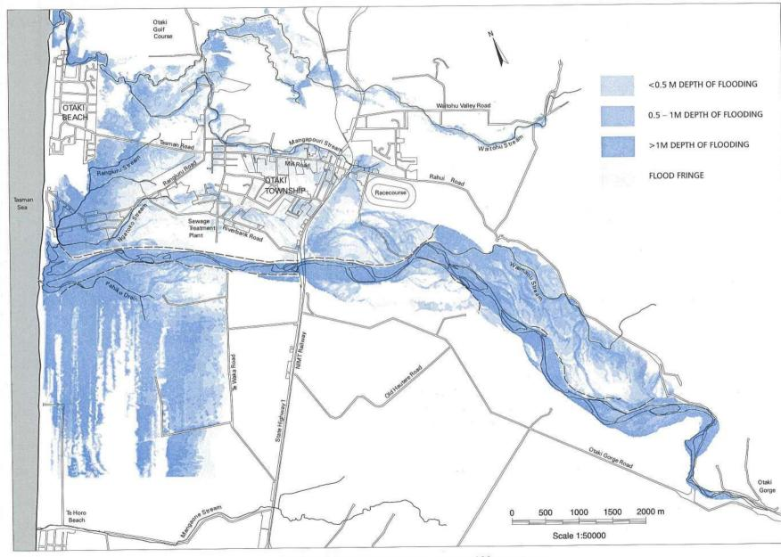
Figure 1: Present extent of flooding in a 100-year flood
