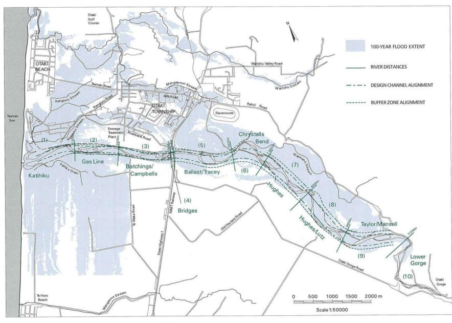
FIGURE 11: CHANNEL ALIGNMENT AND RIVER MANAGEMENT METHODS
