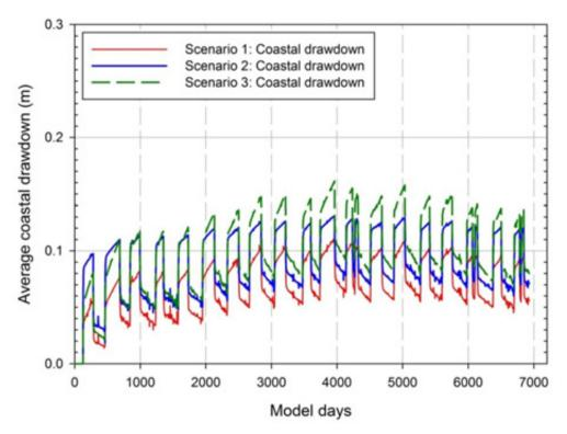
Figure A15: Scenarios 1 to 3 output – coastal aquifer drawdowns in the Waitohu zone resulting from pumping an array of synthetic fully screened wells outside Q1 gravels at 3,000m3/day (Scenario 1), 6,000m3/day (Scenario 2) and 12,000m3/day (Scenario 3) for a 19 year model run
