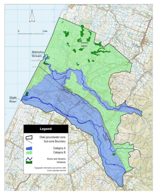
Figure 4.3: Map of the proposed hydraulic connectivity zonation for the Otaki groundwater zone showing the location of significant surface water features and denoting the extent of the Otaki and Waitohu sub-zones
