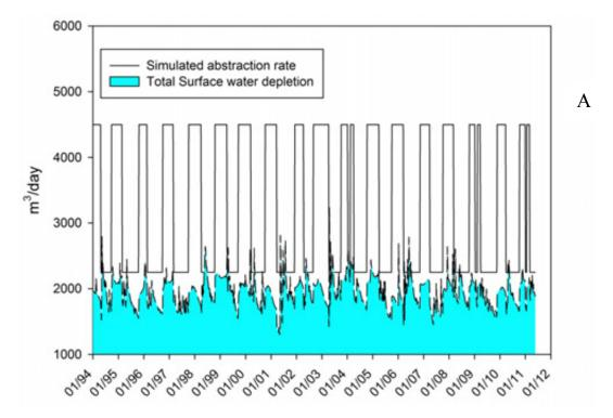
Figure D13: Scenario 4 results – simulated cumulative stream depletion resulting from continuous abstraction (4,500 m³/day summer, 2,250 m³/day winter) over the 1994 to 2012 period
