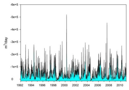
Figure A5: Simulated net natural surface water fluxes to the Waitohu Stream in the Otaki zone when no groundwater abstraction is occurring. The negative fluxes represent flow from groundwater to the stream (i.e. gaining system). This plot shows the net gain over the entire reach of the Waitohu Stream. The plot also shows some positive values during the dry season i.e. net loss from the Waitohu Stream to groundwater.
