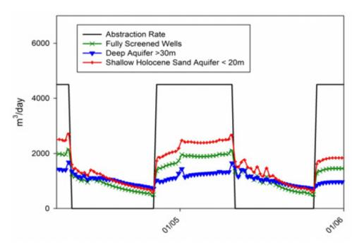
Figure D9: Comparison of cumulative stream depletion resulting from Scenario 1 (abstraction from the shallow Holocene sands), Scenario 2 (abstraction from fully screened bores) and Scenario 3 (abstraction from deeper bores) over the 2004 to 2006 period
