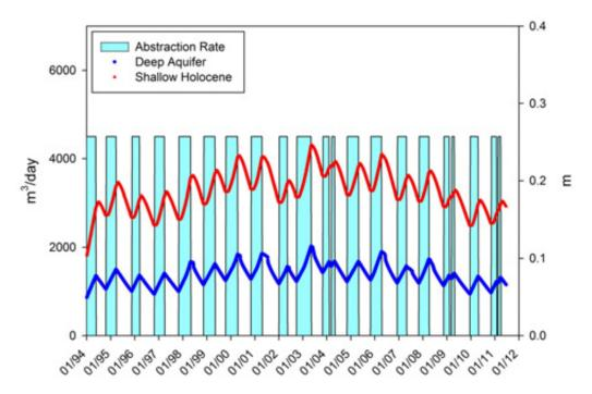
Figure D11: Simulated drawdown resulting from seasonal abstraction at a rate of 4,500 m<sup>3</sup>/day from the shallow Holocene aquifer and deep aquifer respectively between 1994 and 2012
