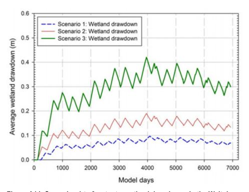
Figure A14: Scenarios 1 to 3 output – wetland drawdowns in the Waitohu zone resulting from pumping an array of synthetic fully screened wells outside Q1 gravels at 3,000m3/day (Scenario 1), 6,000m3/day (Scenario 2) and 12,000m3/day (Scenario 3) for a 19 year model run
