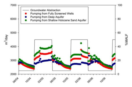
Figure D17: Scenario 4 – surface water depletion (%MALF) resulting from groundwater abstraction from the shallow Holocene sands, deep aquifer and from fully screened wells in the Raumati zone (2004-2006)
