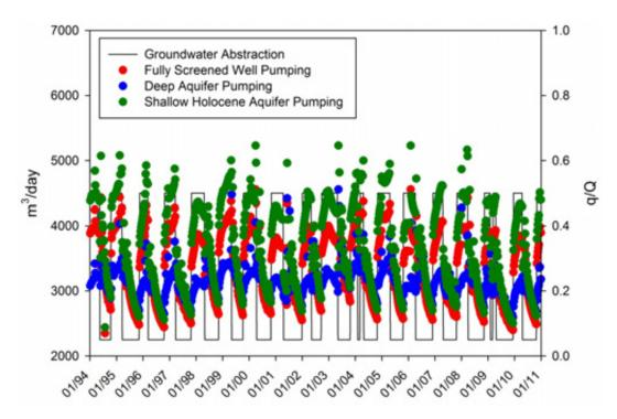
Figure D15: Scenario 4 – surface water depletion resulting from groundwater abstraction from the shallow Holocene sands, deep aquifer and from fully screened wells in the Raumati zone, 1994 to 2012
