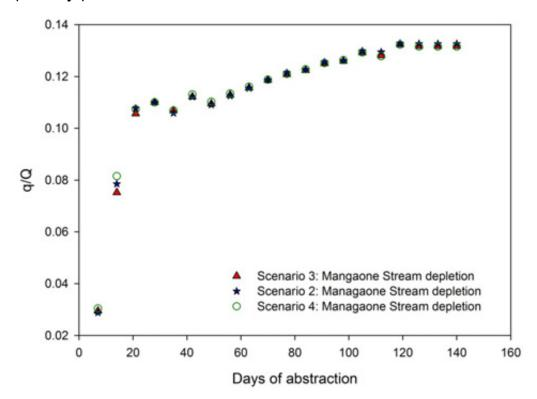
Figure B8: Scenarios 2 to 4 – ratio of surface water depletion (q) to pumping rate (Q) for the Mangaone Stream – abstracting from all the aquifers at 7,500 m<sup>3</sup>/day (Scenario 2), 15,000 m<sup>3</sup>/day (Scenario 3) and 20,000 m<sup>3</sup>/day (Scenario 4)
