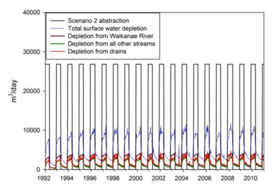
Figure C10: Scenario 2 output – surface water depletion when pumping from Q6 (layers 6 and 7) only of the of the Waikanae zone. Pumping from current consented bores located in the Q6 (> 60m deep) at an abstraction rate of 26,826 m<sup>3</sup>/d.
