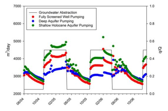
Figure D16: Scenario 4 – surface water depletion resulting from groundwater abstraction from the shallow Holocene sands, deep aquifer and from fully screened wells in the Raumati zone, May 2004 to October 2006
