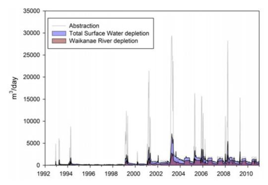
Figure C4: Simulated total surface water depletion resulting from abstraction in the Waikanae zone from all consented bores between 1992 and 2012. The relatively low surface water depletion when compared to groundwater abstraction was due to the short period of high abstractions.
