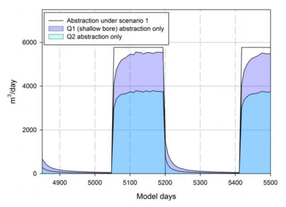
Figure C8: Scenario 1 output – total water depletion in the Waikanae zone from pumping an array of synthetic bores located in the shallow unconfined and semi-confined aquifers in Q1 (ground surface to about 20 m depth) and Q2 (between 20 m to 30 m depth) gravels
