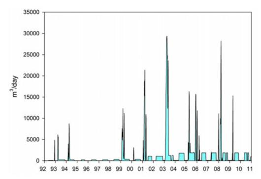
Figure C3: Modelled abstraction in the Waikanae water management zone between 1992 and 2012. The peaks represent the activation of the Waikanae bore field either for water supply or maintenance of the bore field.
