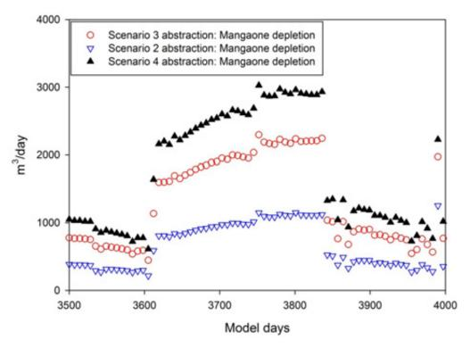
Figure B7: Scenarios 2 to 4 surface water depletion in the Mangaone Stream resulting from pumping an array of synthetic bores located in the three identified aquifers of the Te Horo zone. Abstraction from the aquifer at 7,500m³/day (Scenario 2), 15,000m³/day (Scenario 3) and 20,000m³/day (Scenario 4) extracted from model days 3500 to 4000 from 19 years (6930 days) simulation.
