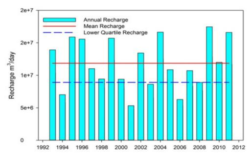
Figure A3: Modelled annual rainfall recharge (1993-2011) for the Waitohu sub-zone between 1992 and 2012. A mean annual recharge of 11.8x10<sup>6</sup>m<sup>3</sup> is indicated as is the lower quartile value of 8.9x10<sup>6</sup>m<sup>3</sup> (dashed line).
