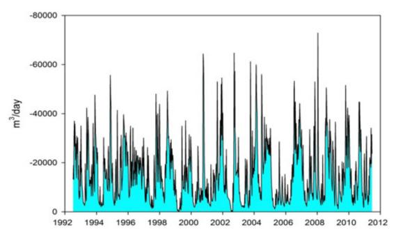
Figure B3: Simulated net natural surface water fluxes to the Mangaone Stream in the Te Horo zone when no groundwater abstraction is occurring. The negative fluxes represent flow from groundwater to the stream (i.e. gaining system). This plot shows the net gain over the entire reach of the Mangaone Stream.
