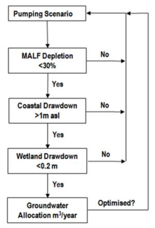
Figure 4.2: Schematic illustration of the iterative modelling process utilised evaluate pumping scenarios and determine groundwater allocation limits
