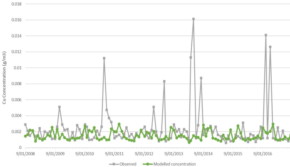
Figure A.19: Comparison of monthly Dissolved Copper concentration at Porirua Stream at Milk Depot
