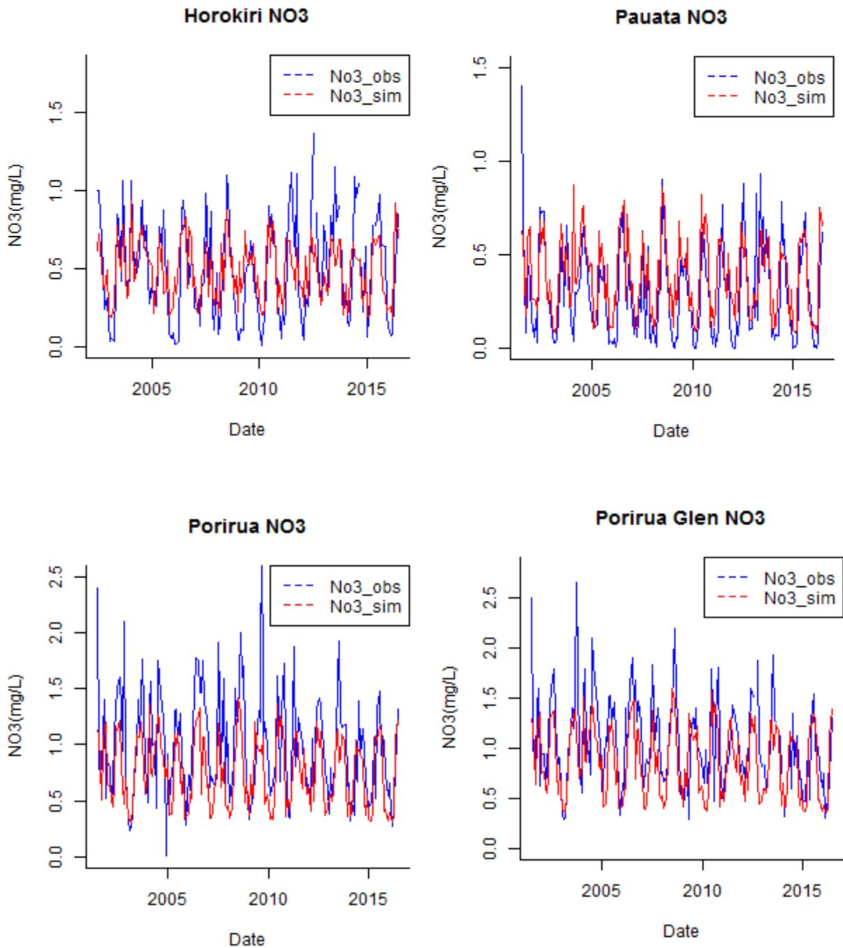
Figure A.10: Comparison of monthly observed and simulated nutrient concentration for Nitrate-Nitrogen (NO<sub>3</sub>-N) at three calibration sites, and the verification site.
