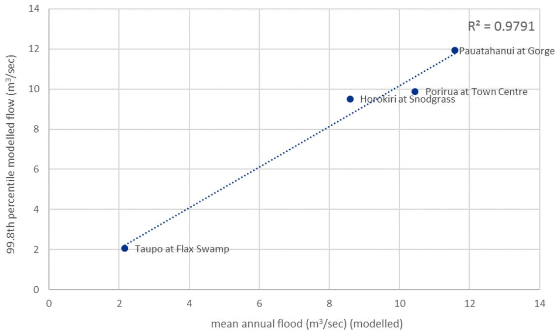
Figure 4.1: Relationship between mean annual flow and 99.8th percentile flow
