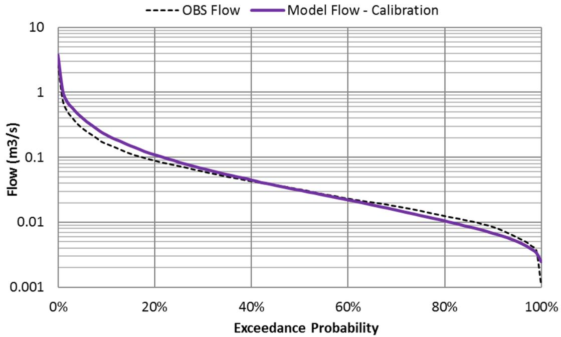
Figure 3.8: Taupo stream at Flax Swamp Calibration Flow Duration Curve
