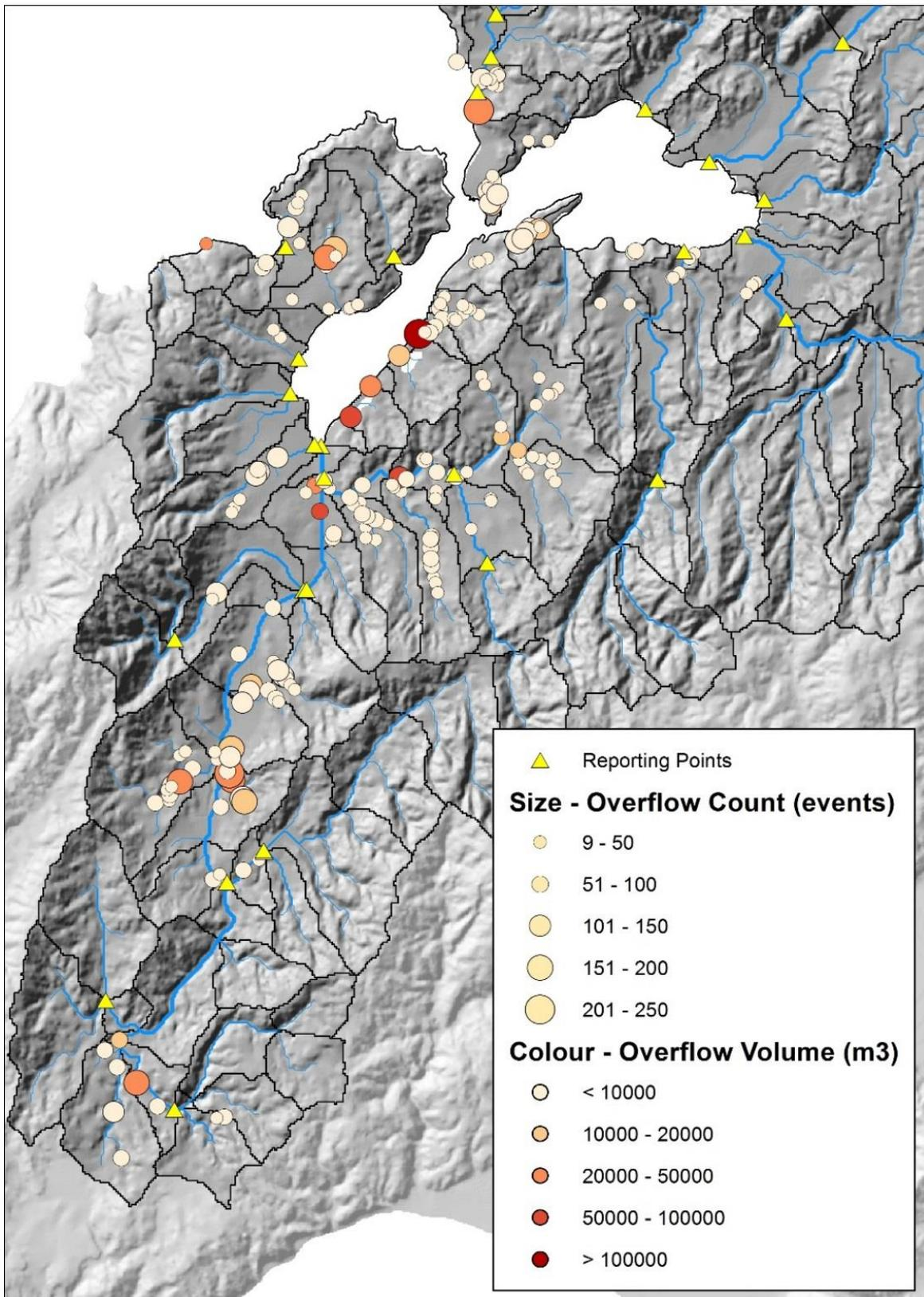
Figure 2.5: Wastewater overflow locations
