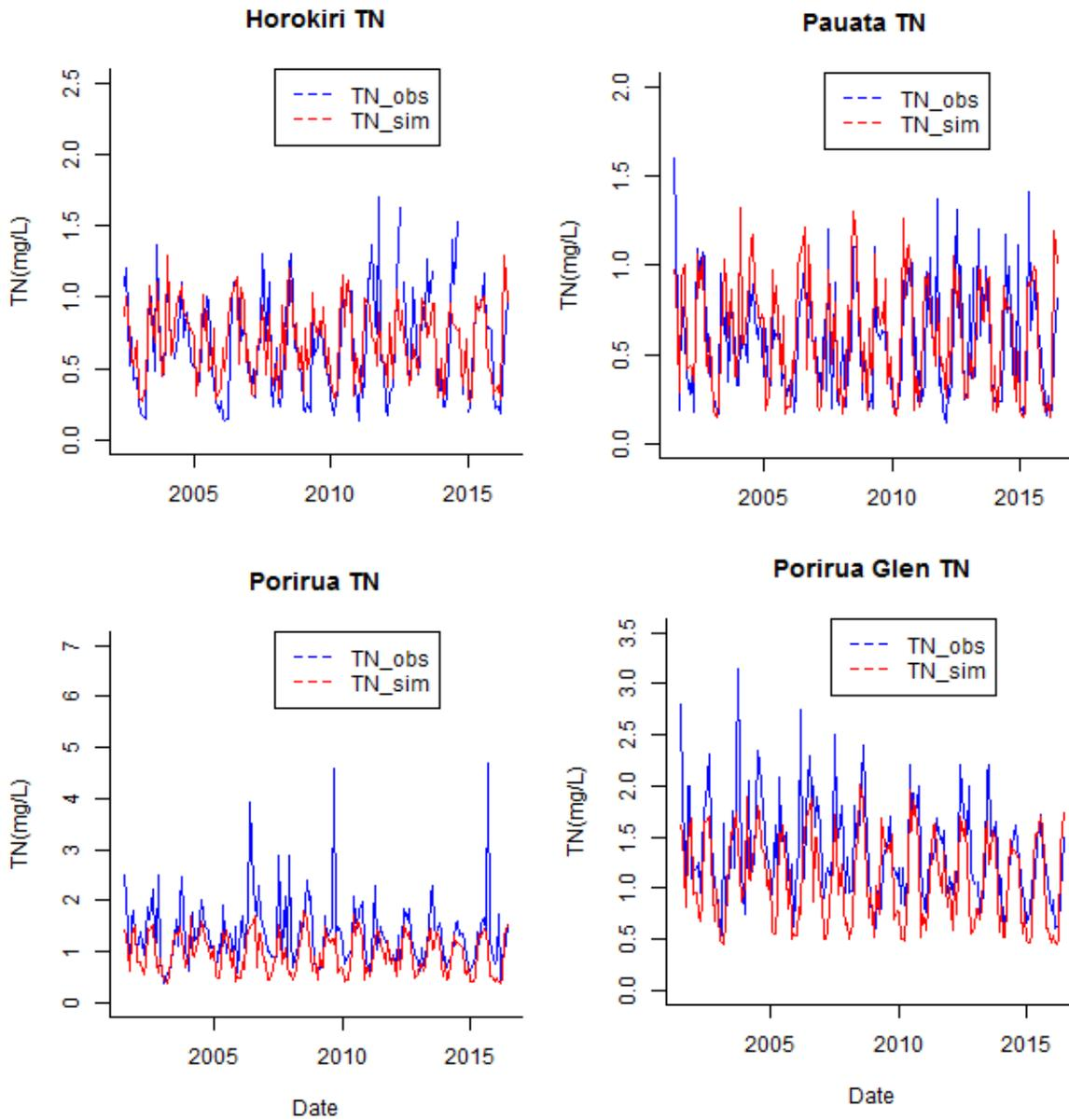
Figure A.9: Comparison of monthly observed and simulated nutrient concentration for Total Nitrogen (TN) at three calibration sites, and the verification site.
