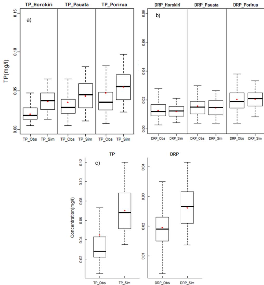
Figure 5.3: Comparison between observed and simulated Box and whisker plot for a) TP and b) DRP for each calibration site, and c) for the Porirua at Glenside verification site.
