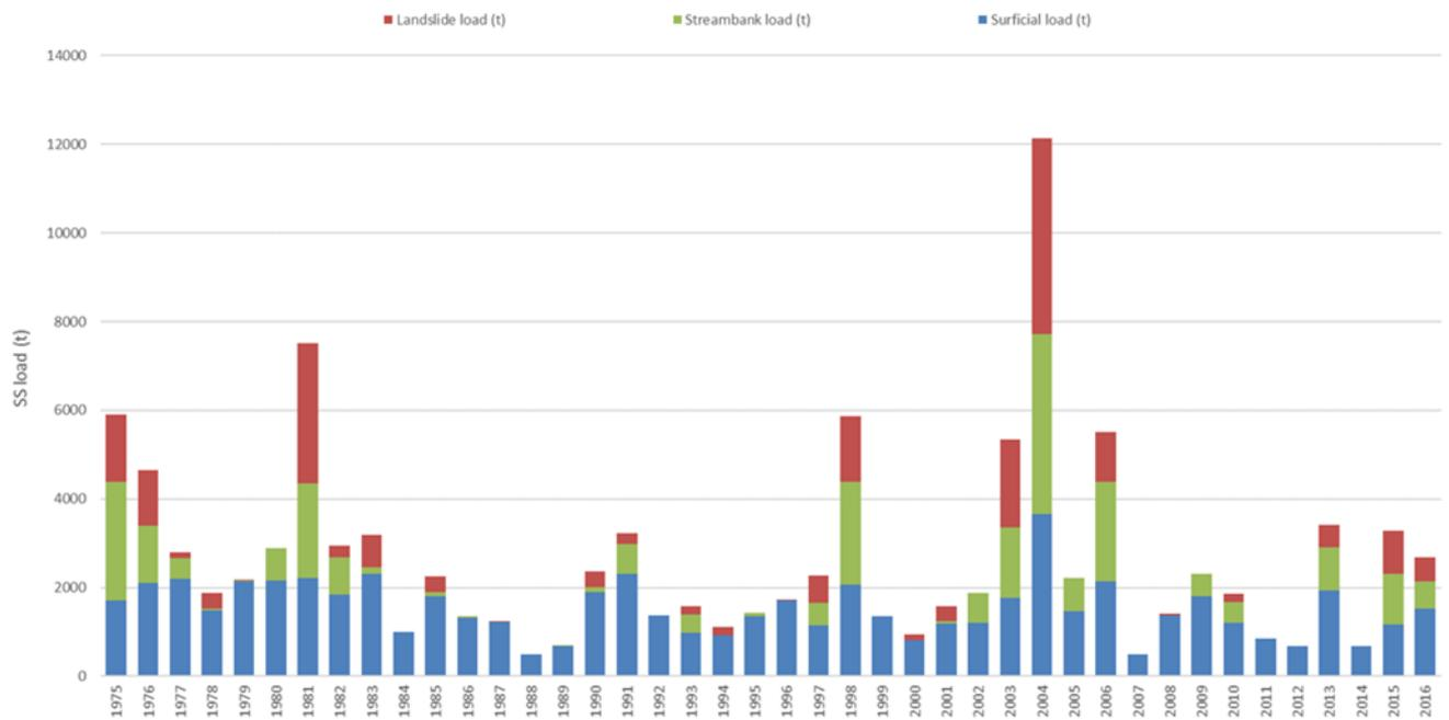
Figure 4.8 Modelled sediment sources for Pauatahanui at Gorge
