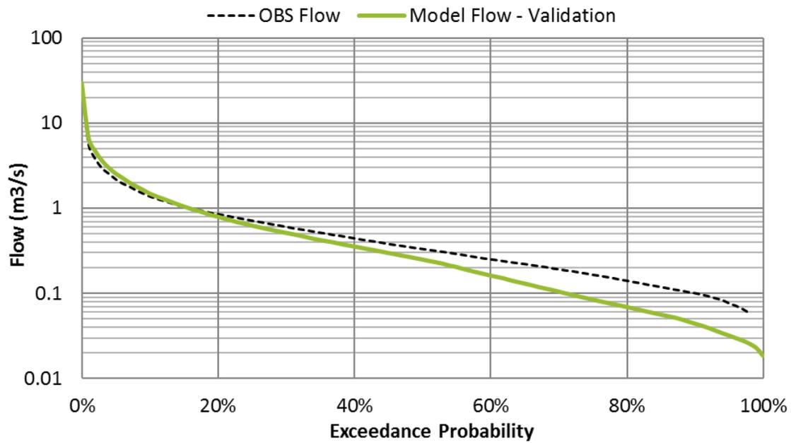
Figure 3.5: Pauatahanui at Gorge Validation Flow Duration Curve
