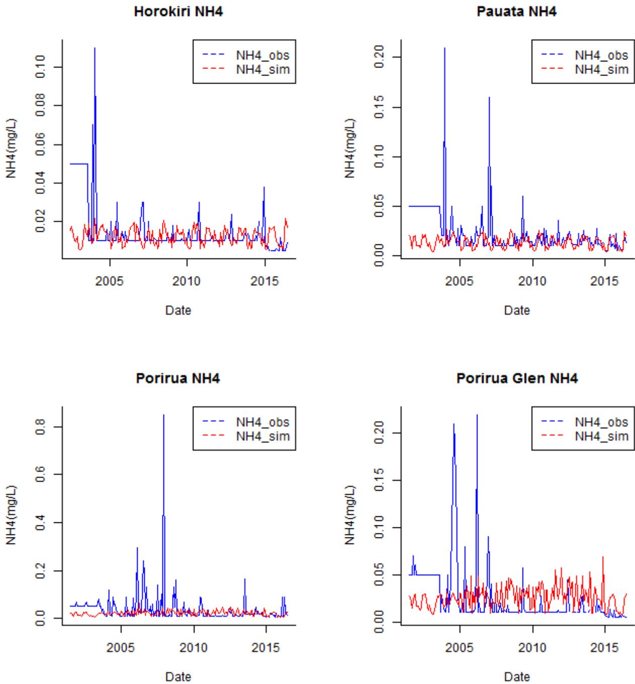
Figure A.11: Comparison of monthly observed and simulated nutrient concentration for Ammoniacal-Nitrogen (NH<sub>4</sub>-N) at three calibration sites, and the verification site.
