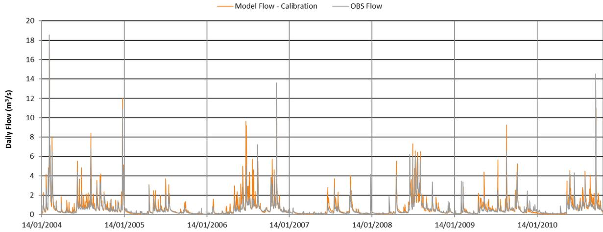
Figure A.1: Horokiri at Snodgrass Flow – Calibration period
