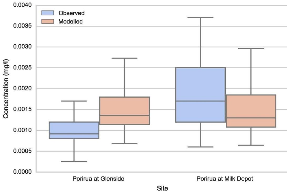
Figure 6.4: Boxplot comparison for Dissolved Copper concentration at two calibration sites
