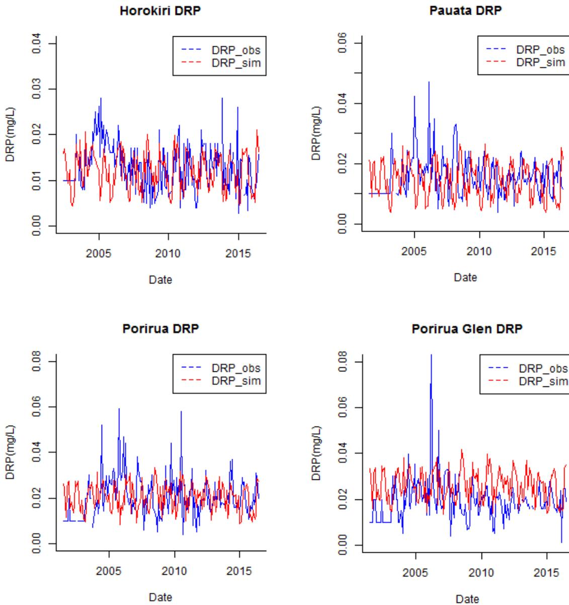
Figure A.13: Comparison of monthly observed and simulated Dissolved Reactive Phosphorus (DRP) concentrations at each calibration site and the verification site.
