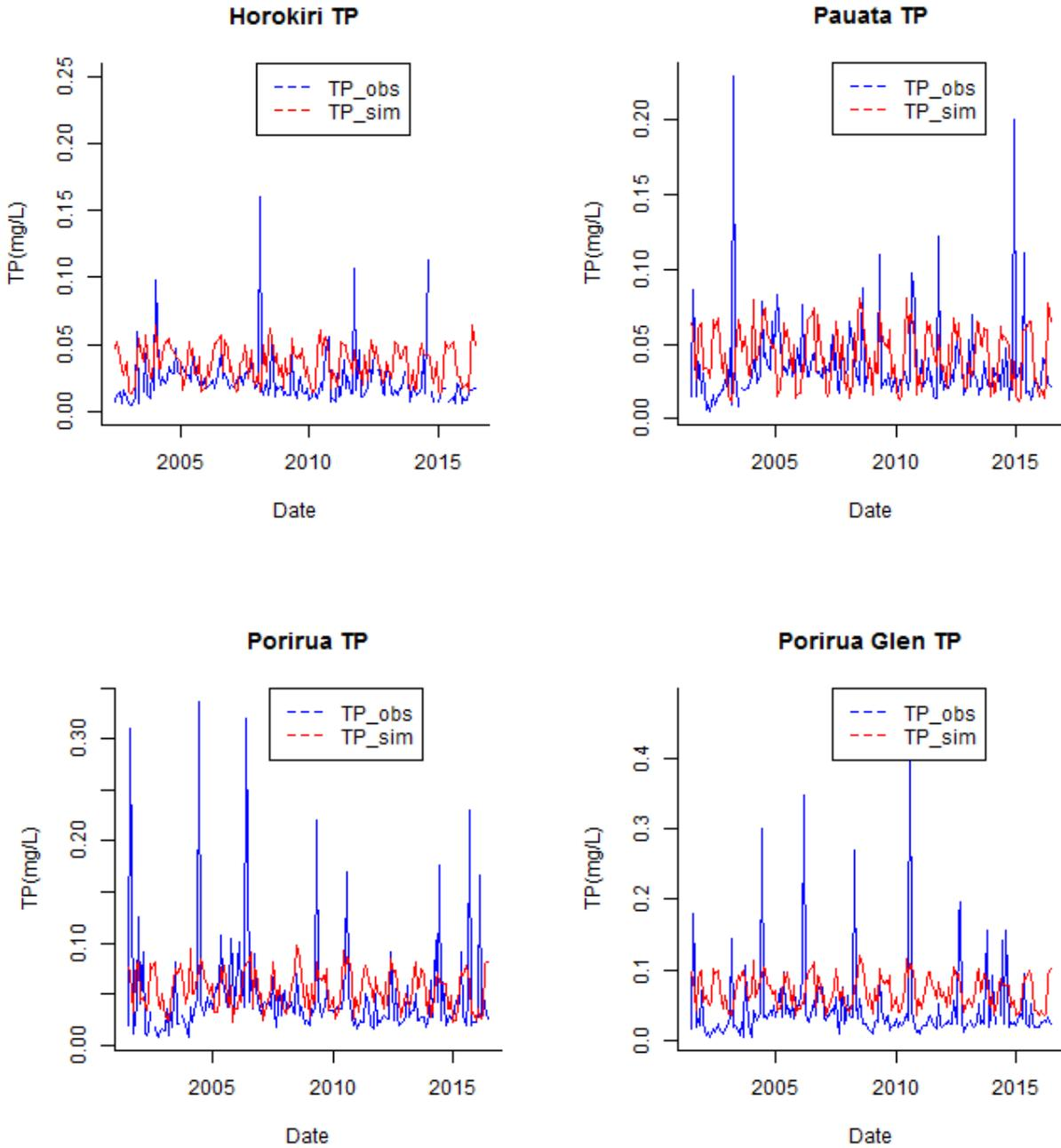
Figure A.12: Comparison of monthly observed and simulated total phosphorus (TP) concentrations at each calibration site and the verification site.
