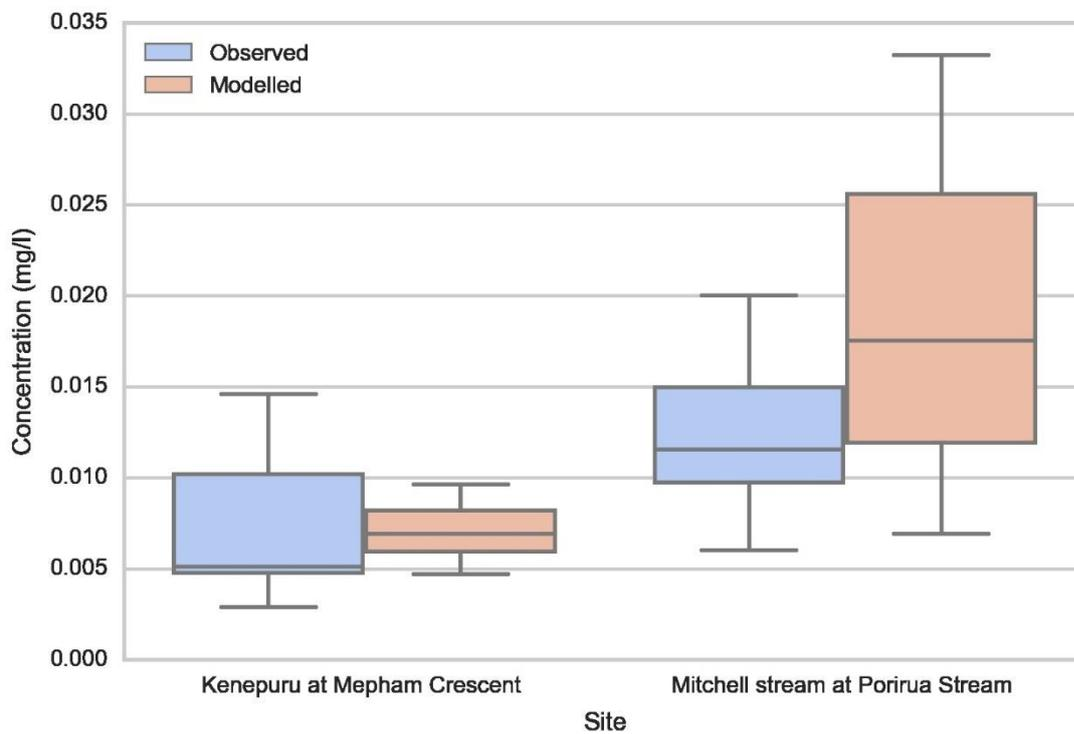
Figure 6.3 Boxplot comparison for Dissolved Zinc concentration at two validation sites.
