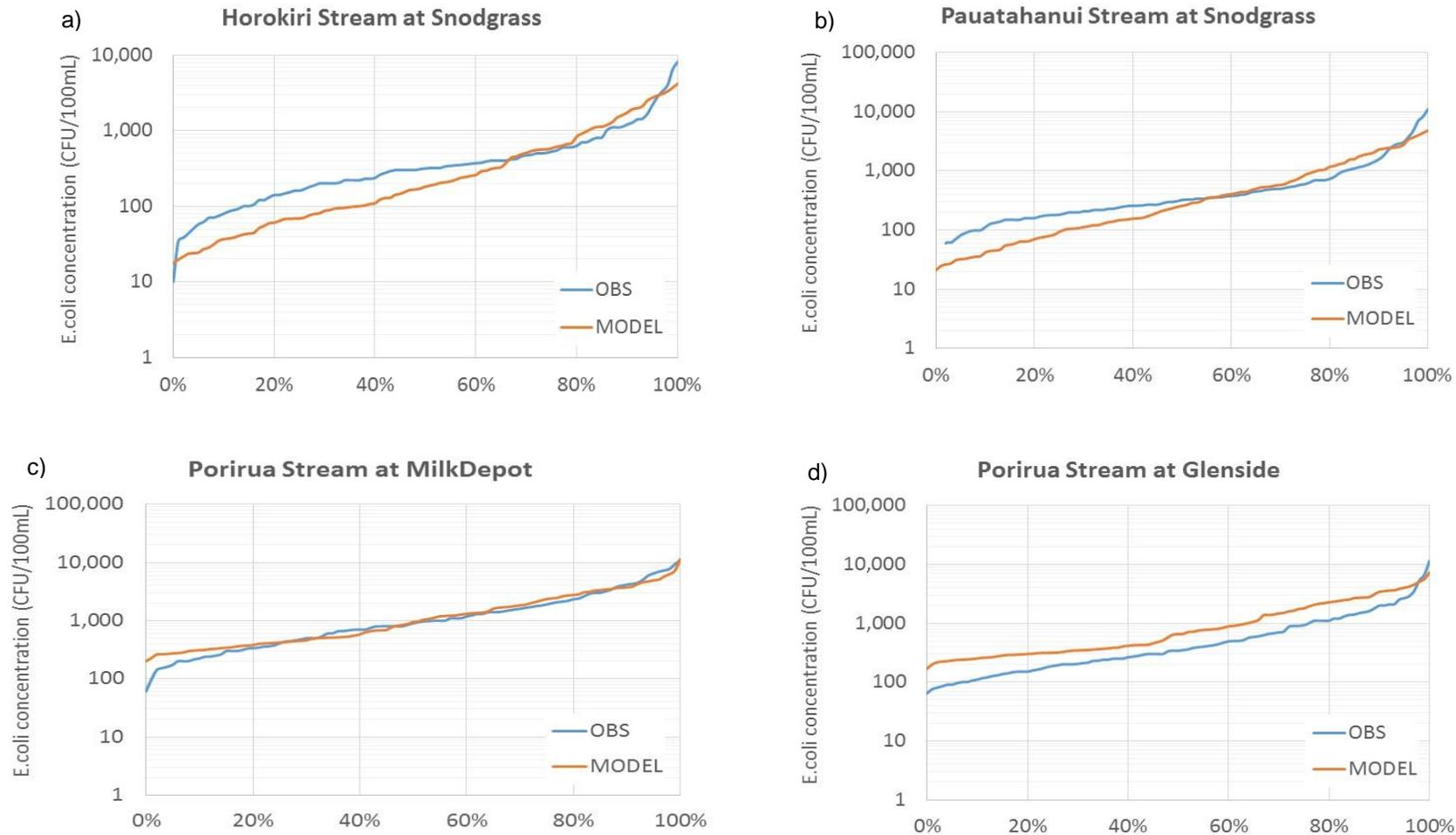
Figure 7.2: Exceedance curve for observed and simulated *E. coli* at: a) Horokiri Stream at Snodgrass; b) Pauatahanui Stream at Elmwood Bridge; c) Porirua Stream at Milk Depot and d) Porirua Stream at Glenside Overhead Cables.
