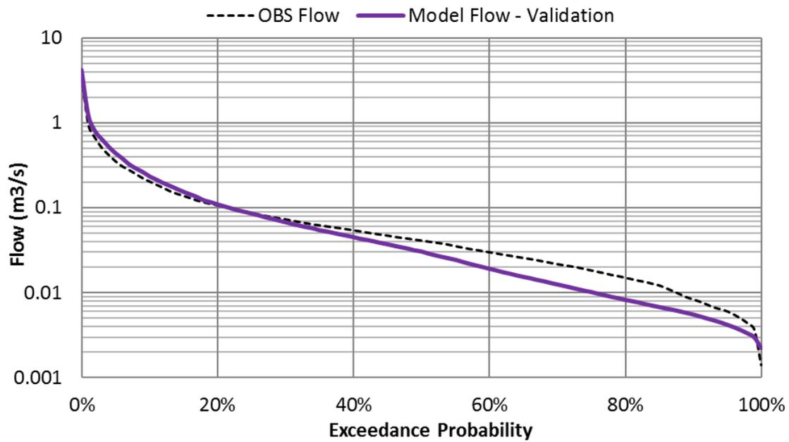
Figure 3.9: Taupo stream at Flax Swamp Validation Flow Duration Curve
