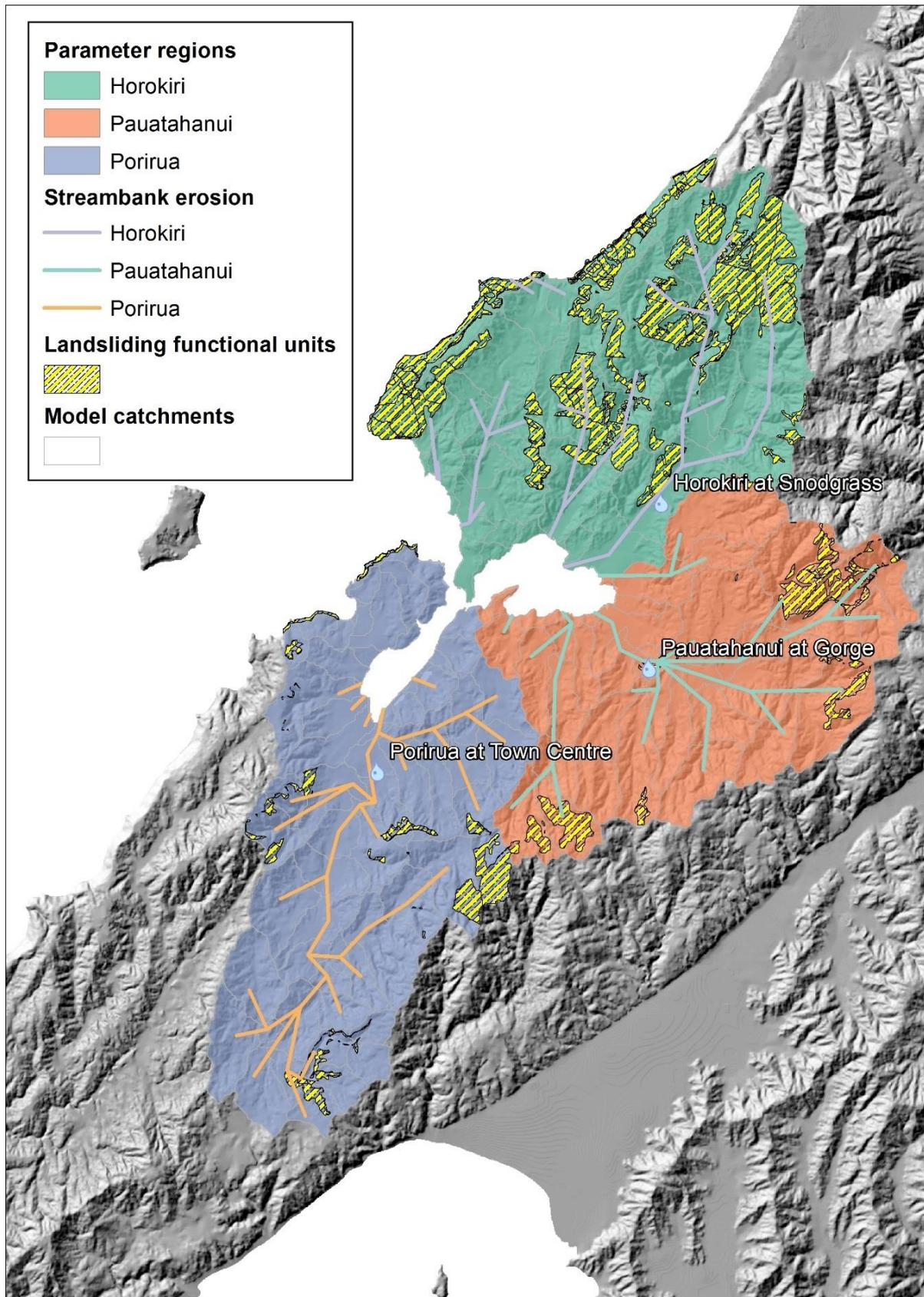
Figure 4.2: Erosion model overview and parameter regionalisation
