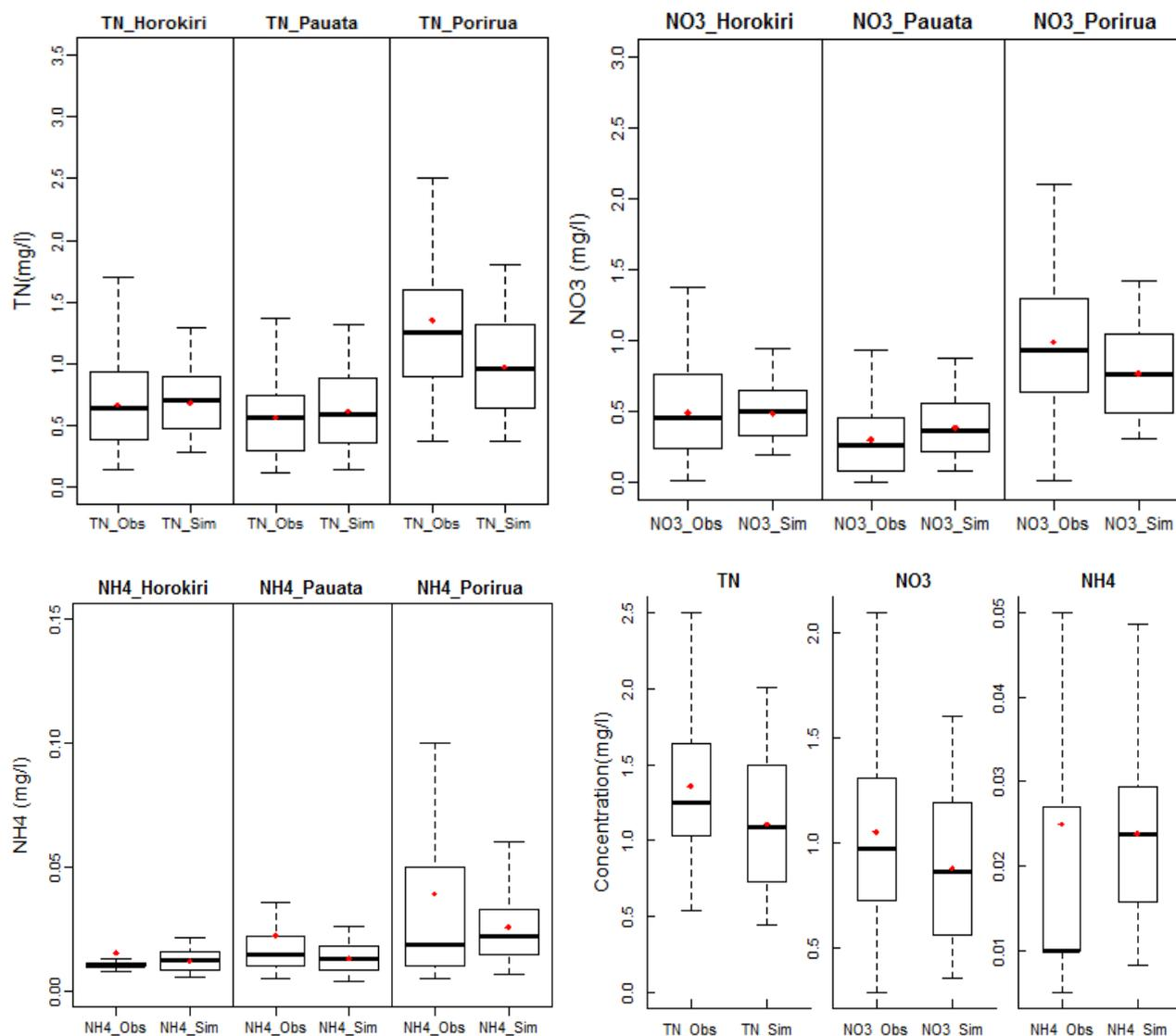
Figure 5.2: Comparison between monthly observed and simulated Box and whisker plot for a) TN, b) NO<sub>3</sub>-N and c) NH<sub>4</sub>-N for each calibration site; and d) for the Porirua at Glenside verification site.
