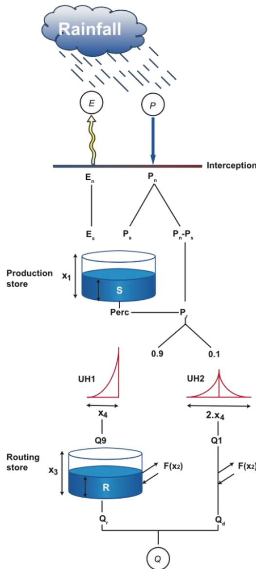
Figure 3.1: GR4J Rainfall-Runoff schematic (eWater, 2015)
