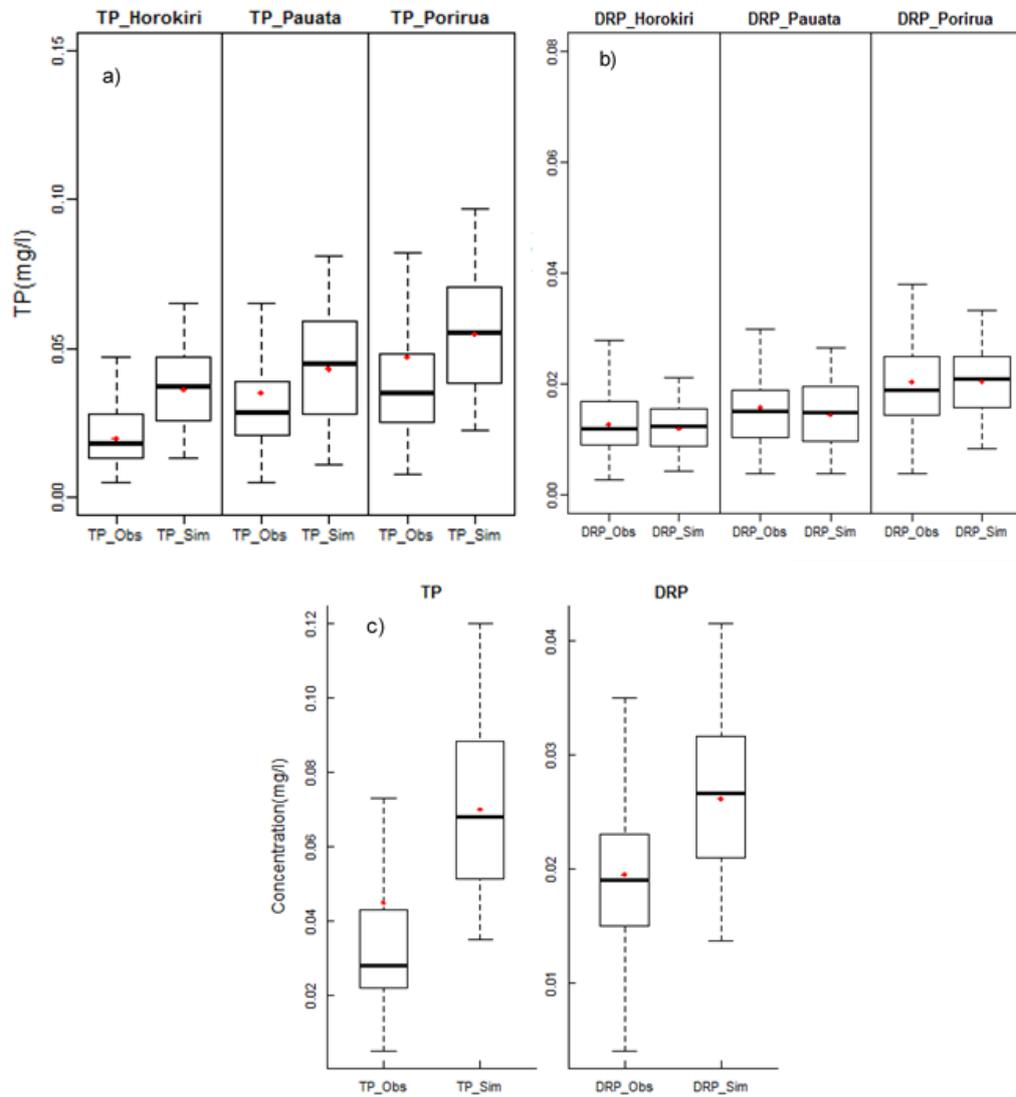
Figure 5.3: Comparison between observed and simulated Box and whisker plot for a) TP and b) DRP for each calibration site, and c) for the Porirua at Glenside verification site.
