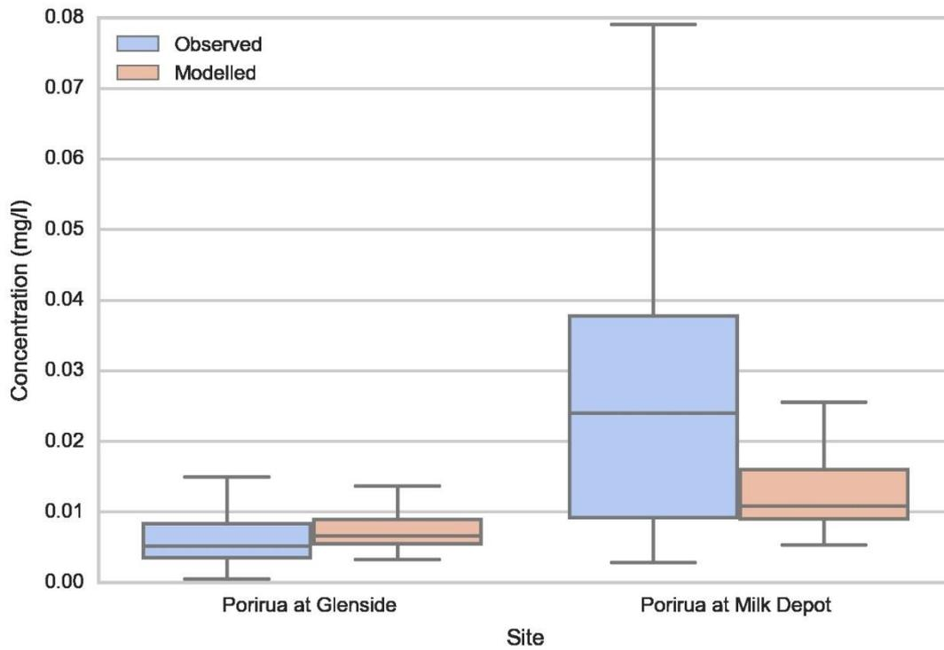
Figure 6.2: Boxplot comparison for Dissolved Zinc concentration at two calibration sites.
