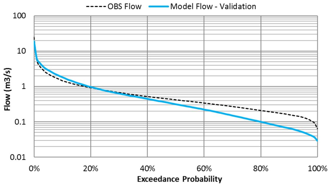
Figure 3.7: Porirua at Town Centre Validation Flow Duration Curve
