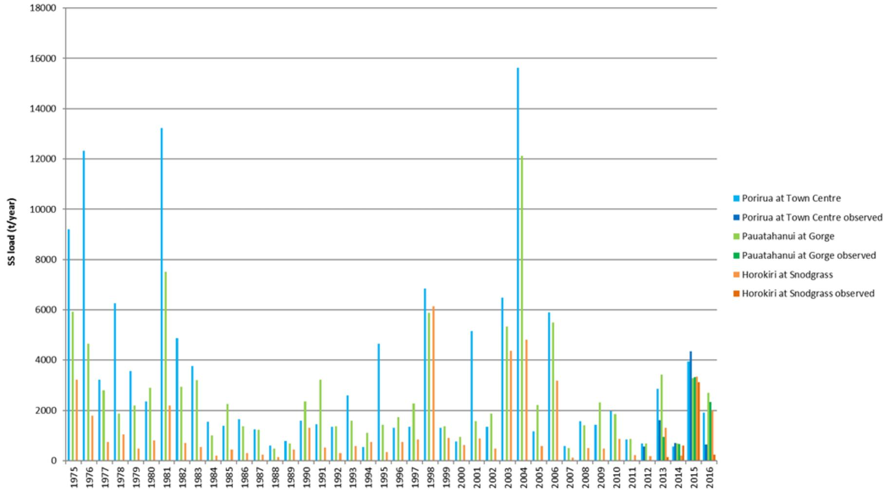
Figure 4.6: Modelled and observed annual sediment loads (t/year) (observed data incomplete – see Table 4.4)
