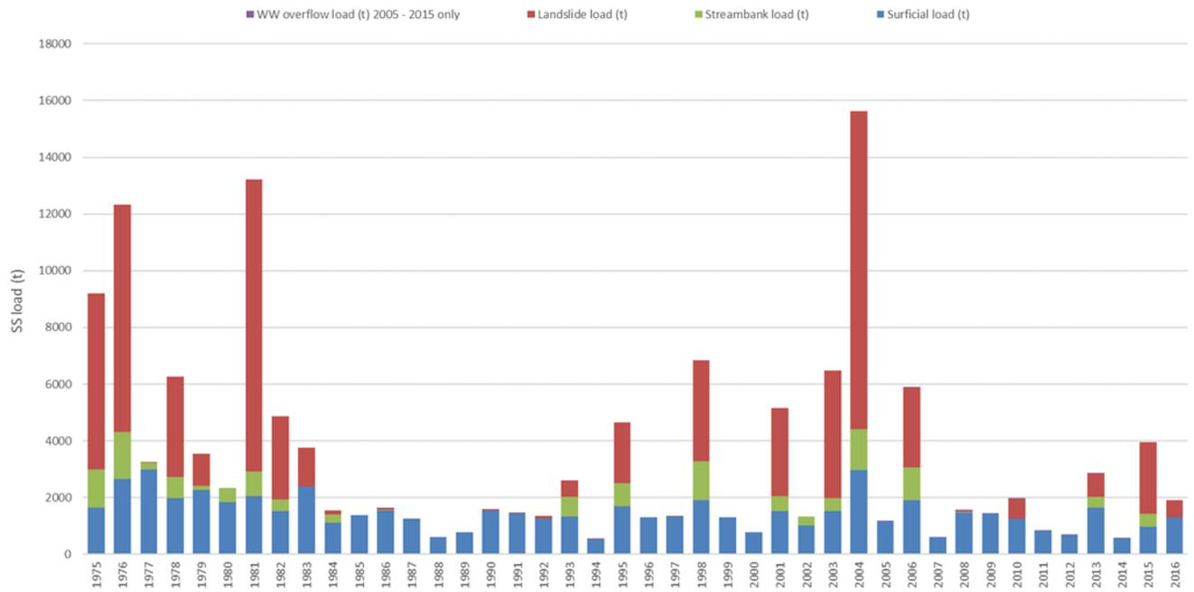
Figure 4.7: Modelled sediment sources for Porirua at Town Centre
