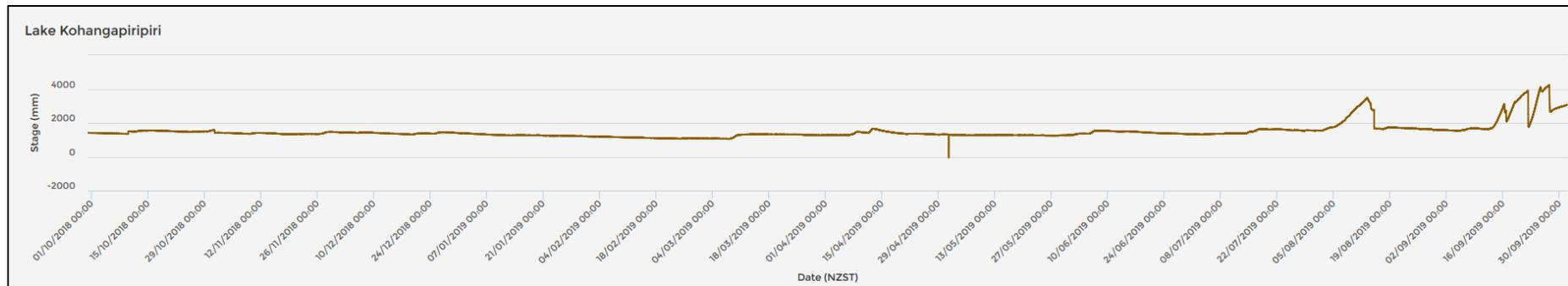
**Figure 3.** Hydrograph of Lake Kohangapiripiri from Oct 2018 to Sept 2019, showing a pattern typical of seepage discharge, with no cutting through of the gravel barrier bar. Data are from the Greater Wellington Regional Council website ([http://graphs.gw.govt.nz/?siteName=Lake Kohangapiripiri&dataSource=Stage](http://graphs.gw.govt.nz/?siteName=Lake%20Kohangapiripiri&dataSource=Stage)).
