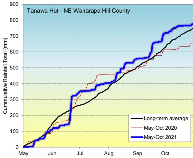
*The Tanawa Hut rain gauge in the Wairarapa Coast area shows a steep increase due to very wet conditions during June before flattening off thanks to a dry July*
