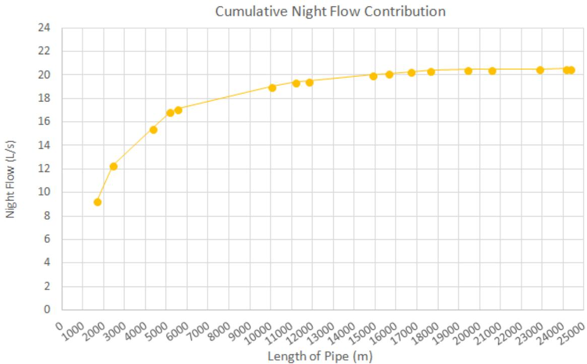
Figure 4 Cumulative Night Flow Contributions (Pipe Length and Flow Rate)
