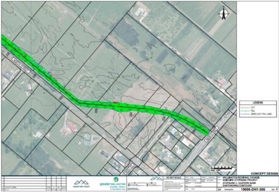
Figure 105: Example of Mapped Path of Stopbank – CF Projects Limited.
