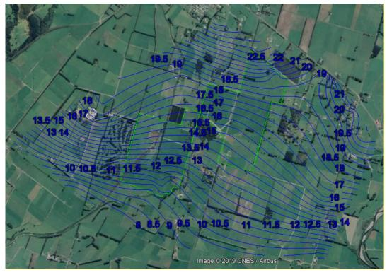
Figure 4 Interpreted Water Table Elevation Plan (m RL) Nov - Dec 2018
