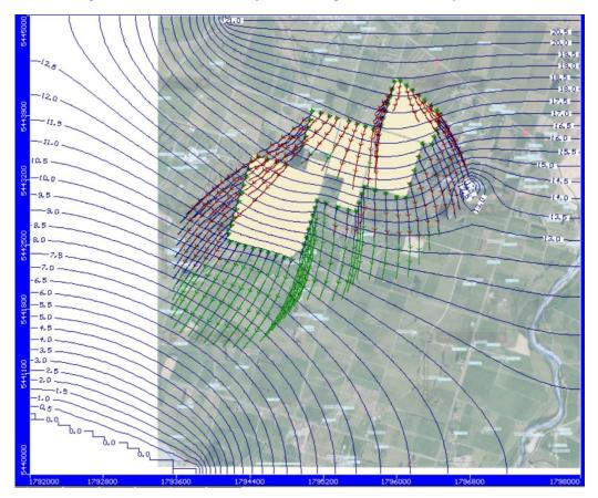
Figure 9 Flow Path Lines Showing 5 Year Travel Envelope
