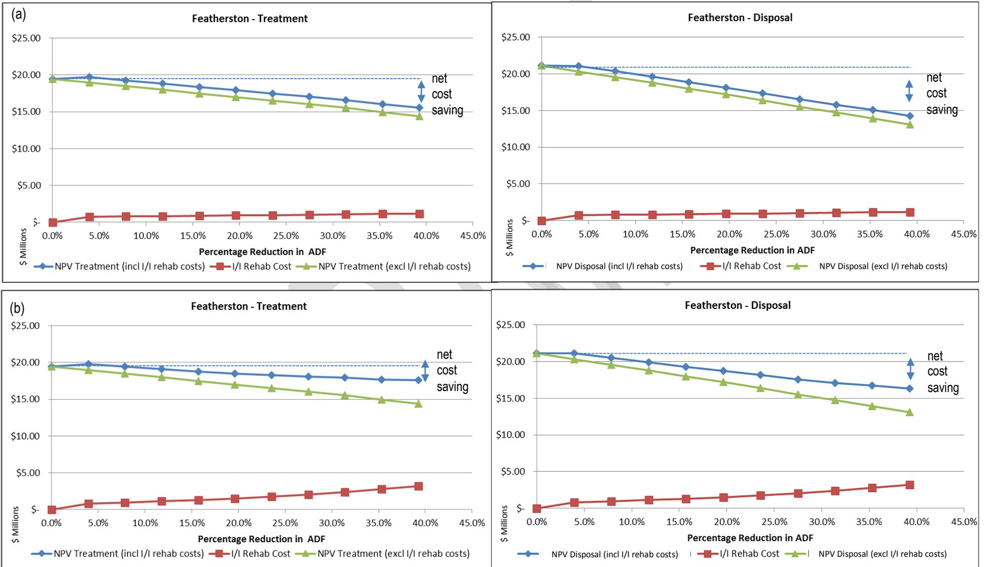
Figure 25: Effect of I/I reduction on NPV for Featherston High Rate Treatment & Land Disposal options (a) 5% and (b) 30% of network requiring rehabilitation
