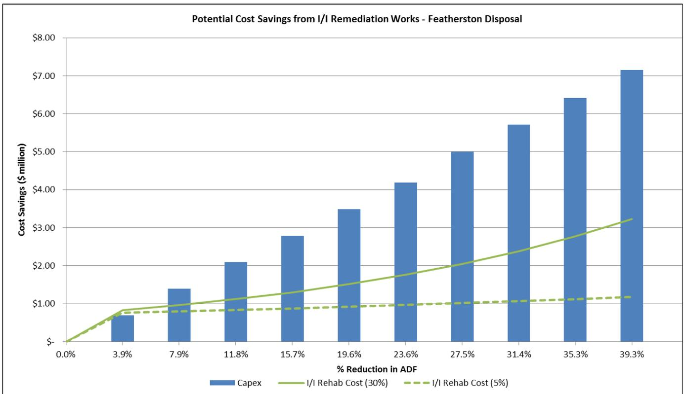
Figure 24: Potential capex savings from Featherston I/I Works – (a) Treatment and (b) Disposal
