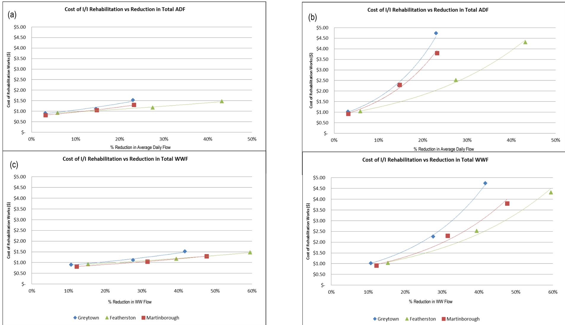
Figure 23: Indicative Cost (\$millions) of I/I rehabilitation vs reduction in ADF and WWF for (a & c) 5% and (b & d) 30% of network requiring rehabilitation
