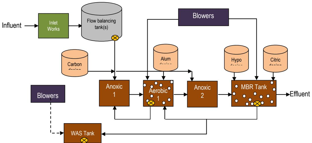
Figure 14: Process flow diagram for membrane bioreactor process
