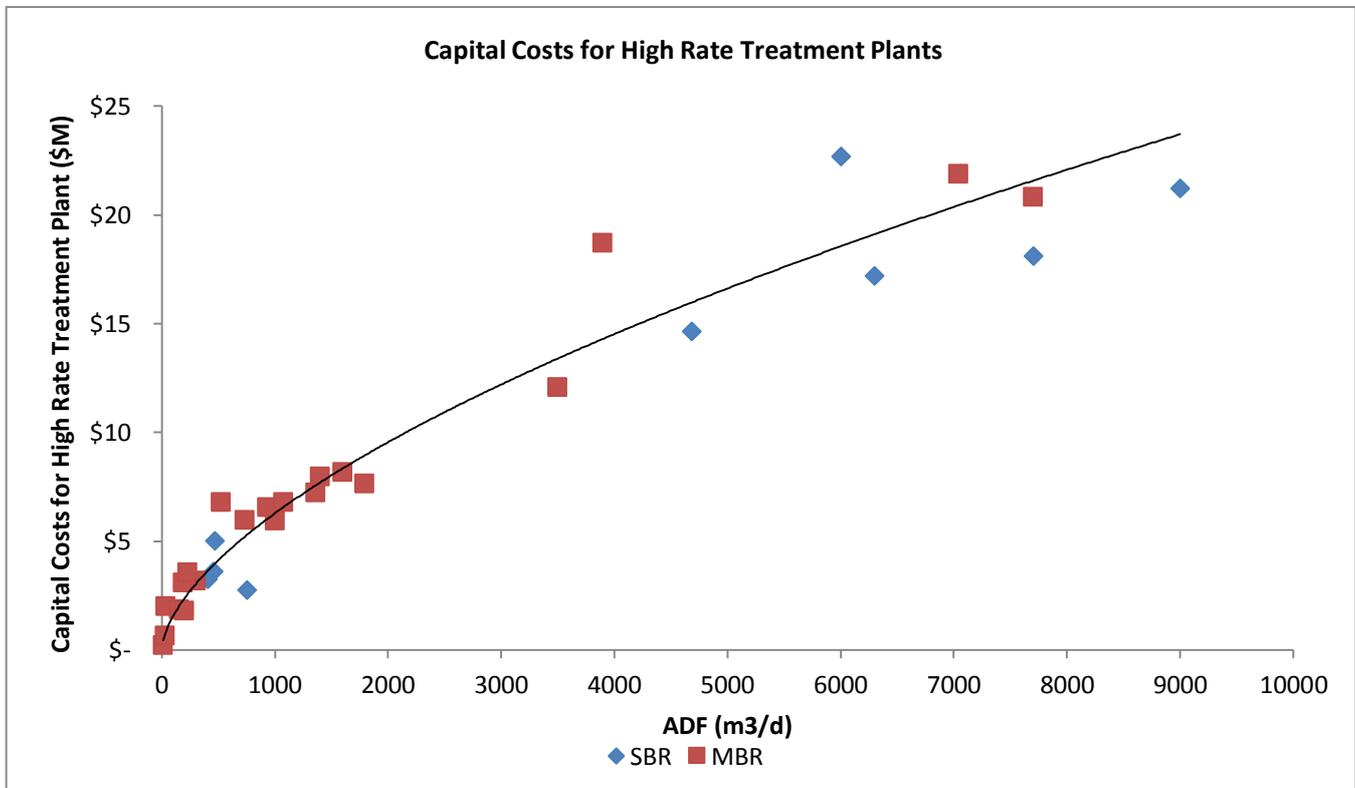
Figure 16: Cost curve for high rate treatment plant capex cost
