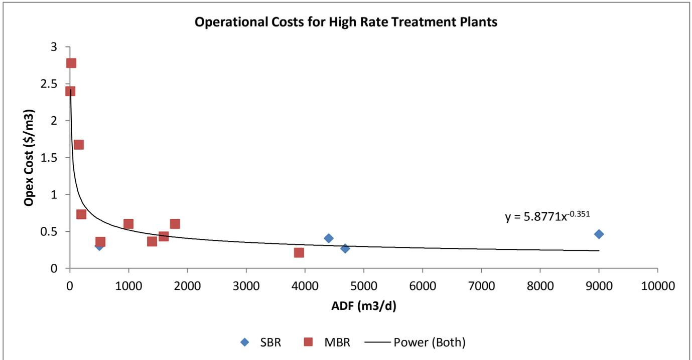
Figure 17: Cost curve for high rate treatment plant opex cost
