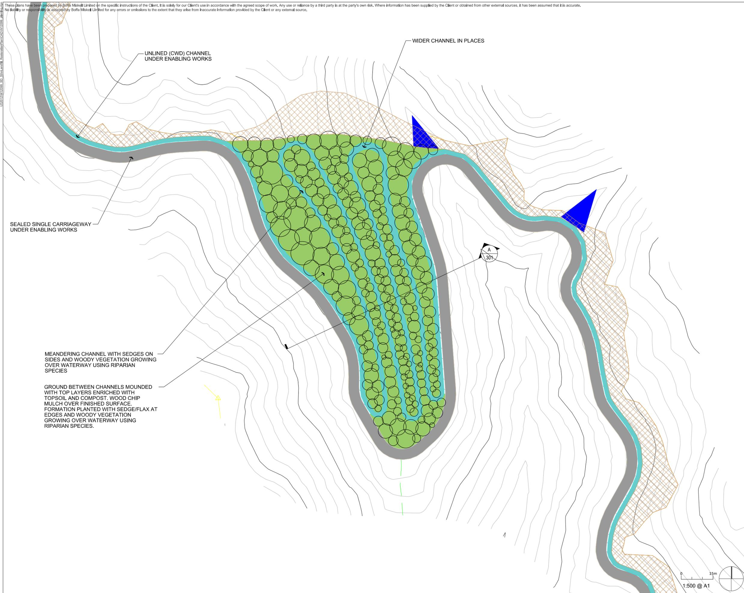
UNLINED (CWD) CHANNEL UNDER ENABLING WORKS
