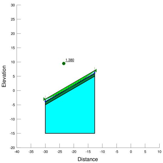
Model: Mohr-Coulomb Unit Weight: 22 kN/m³ Cohesion: 15 kPa Phi: 35 ° Piezometric Line: 1
