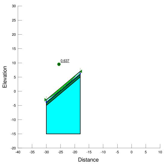
Model: Mohr-Coulomb Unit Weight: 22 kN/m<sup>3</sup> Cohesion: 15 kPa Phi: 35 ° Piezometric Line: 1
