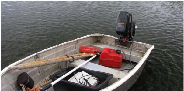
Figure 1. A small aluminium dinghy was used to survey rivers. The long-cabled salinity sensor can be seen coiled in the black plastic box.
