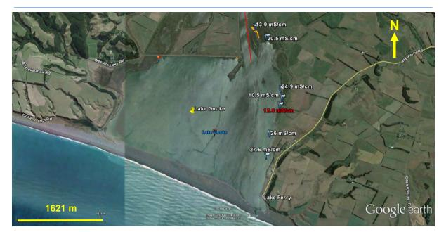
**Figure 22b.** Conductivity of waters in Lake Onoke illustrating the lower readings in the vicinity of freshwater seeps along the north and eastern shoreline. Red line = Ruamahanga River course. Red value is conductivity in an occluded lagoon formed by a historic old braid, separated from the lake by a gravel bund.
