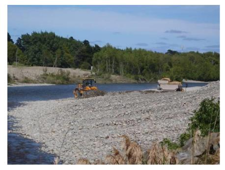
Front-end loader loading an off-road dumper truck
