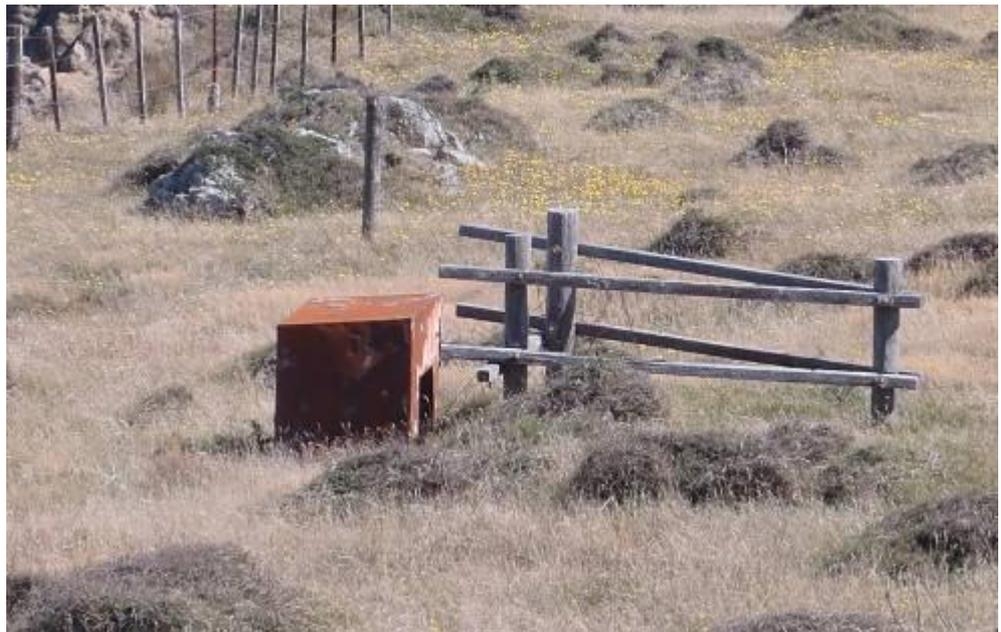
Figure 24: The winch. This has a wing fence surrounding it to protect it from stock.
