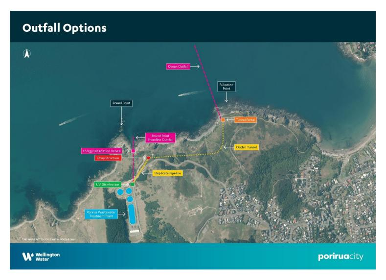
Figure 1., continued. Location of the alternative outfall options at Round Point (option 3) and offshore from the existing outfall (option 5b).
