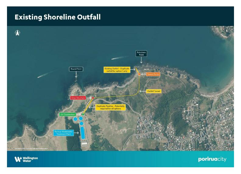
Figure 1. Location of the three outfall options. Location of the existing outfall (option 1) at Rukutane Point.
