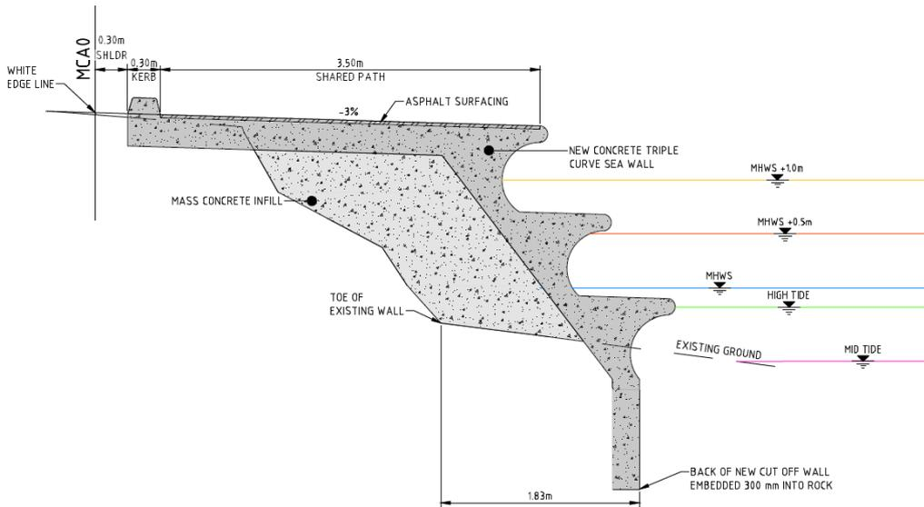
Figure 3-5: Triple curved concrete wall
