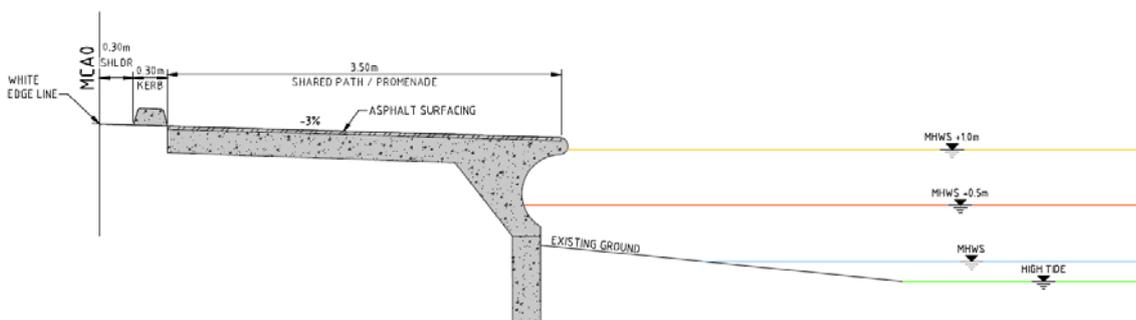
Figure 3-3: Single curved concrete seawall
