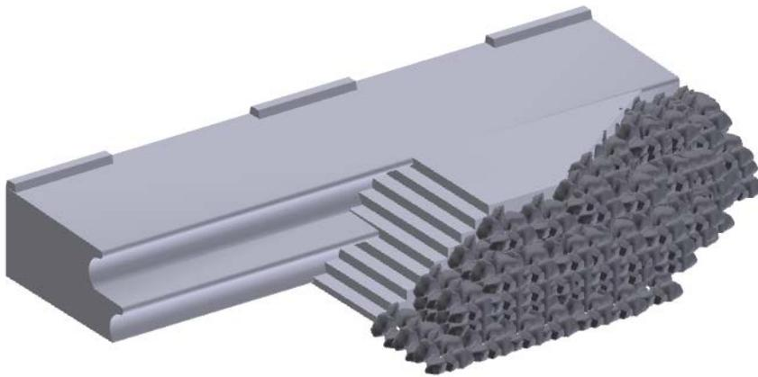
Figure 3-7: Parallel Access Steps on Double Curve Wall with Rock Rip Rap
