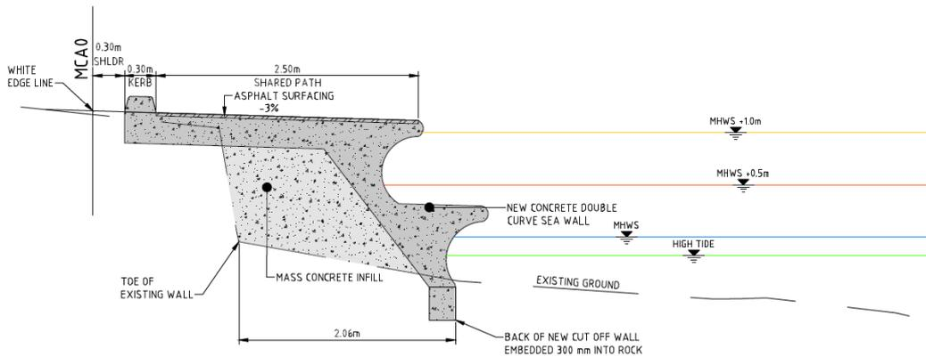
Figure 3-4: Double curved concrete wall
