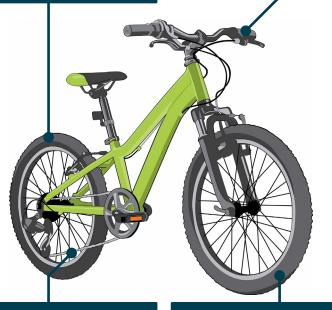
Chain – check the chain has clean oil on it and can move freely. The chain should look black or silver, not rusty. A little oil should come off if you touch it. If dirty oil has built up, clean that off first before adding more oil. Direction – with the front wheel "parked" between your legs, try to turn the handlebars firmly. The wheel should turn with the handlebars, and the handlebars shouldn't feel loose or wobbly.
