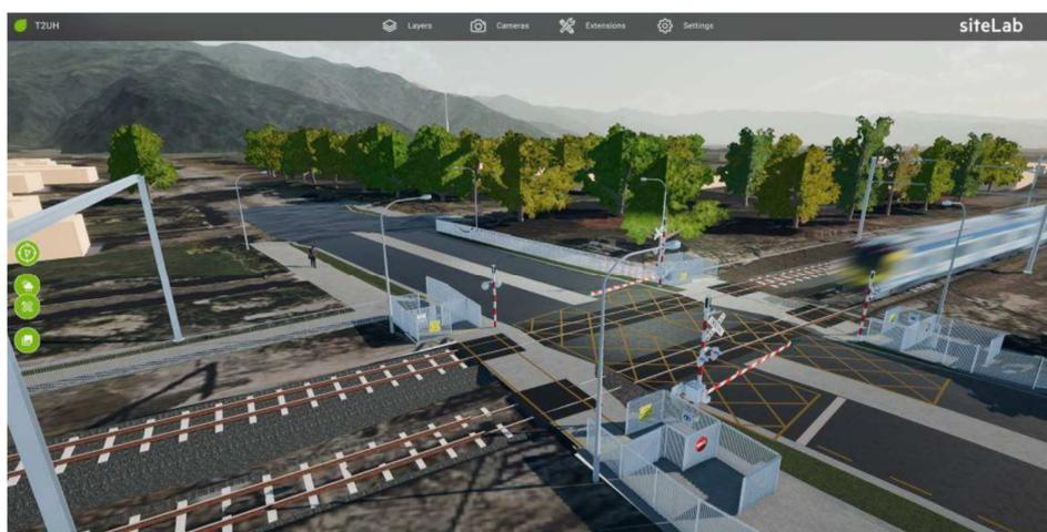
**Image taken from Digital Engineering 3D model of Wallaceville level crossing**
