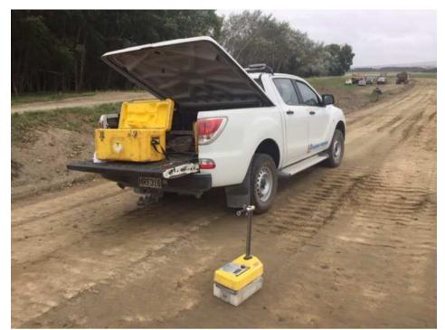
Consultant operating nuclear densometer for compaction testing on the new stopbank
