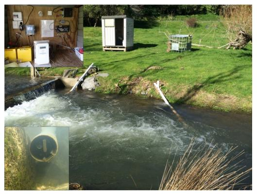
Figure A2.2: Horokiri Stream at Snodgrass site with insets of the SC-200 control unit and logger setup (top left), and primary in-stream turbidity sensor (bottom left inset and pipe near weir). The backup OBS-3 turbidity sensor (not shown) is attached to the outside of the pipe near weir
