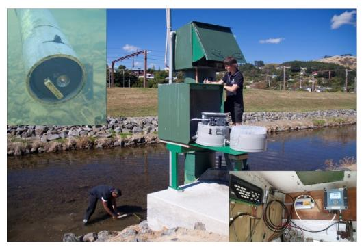
Figure A2.1: Porirua Stream at Town Centre site. Top left inset: Turbidity sensor in the stream with lens and wiper showing. Bottom right inset: SC-200 control unit (top right) and logger (top left) setup
