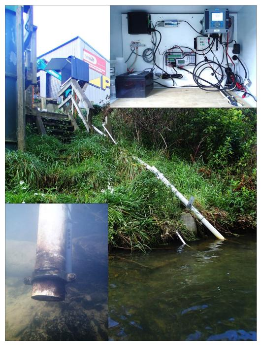
Figure A2.3: Pauatahanui Stream at Gorge site with insets of the SC-200 control unit and logger setup (top right) and in-stream turbidity sensor with auto-sampler intake hose attached to sensor housing (bottom left)
