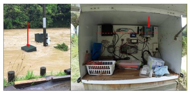
Figure 3.10: Pauatahanui Stream at Gorge site during 14 November 2016 flood (left) showing station box with turbidity instrumentation (right) being flooded; dashed line is water level at peak of flood
