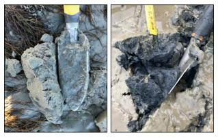
Examples of well oxygenated sandy sediment with aRPD >150mm (left) and poorly oxygenated muddy sediment with aRPD <5mm (right).
