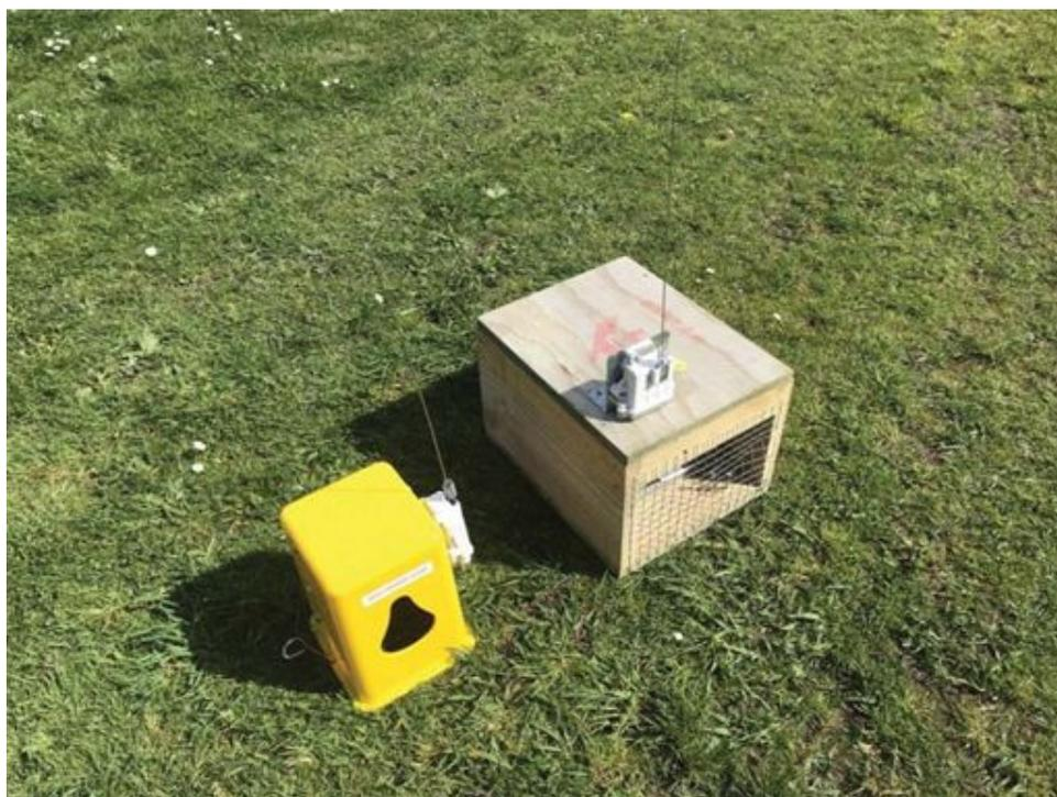
Image 6. Celium electronic wireless sensor nodes attached to Timms trap and DOC250 trap.
