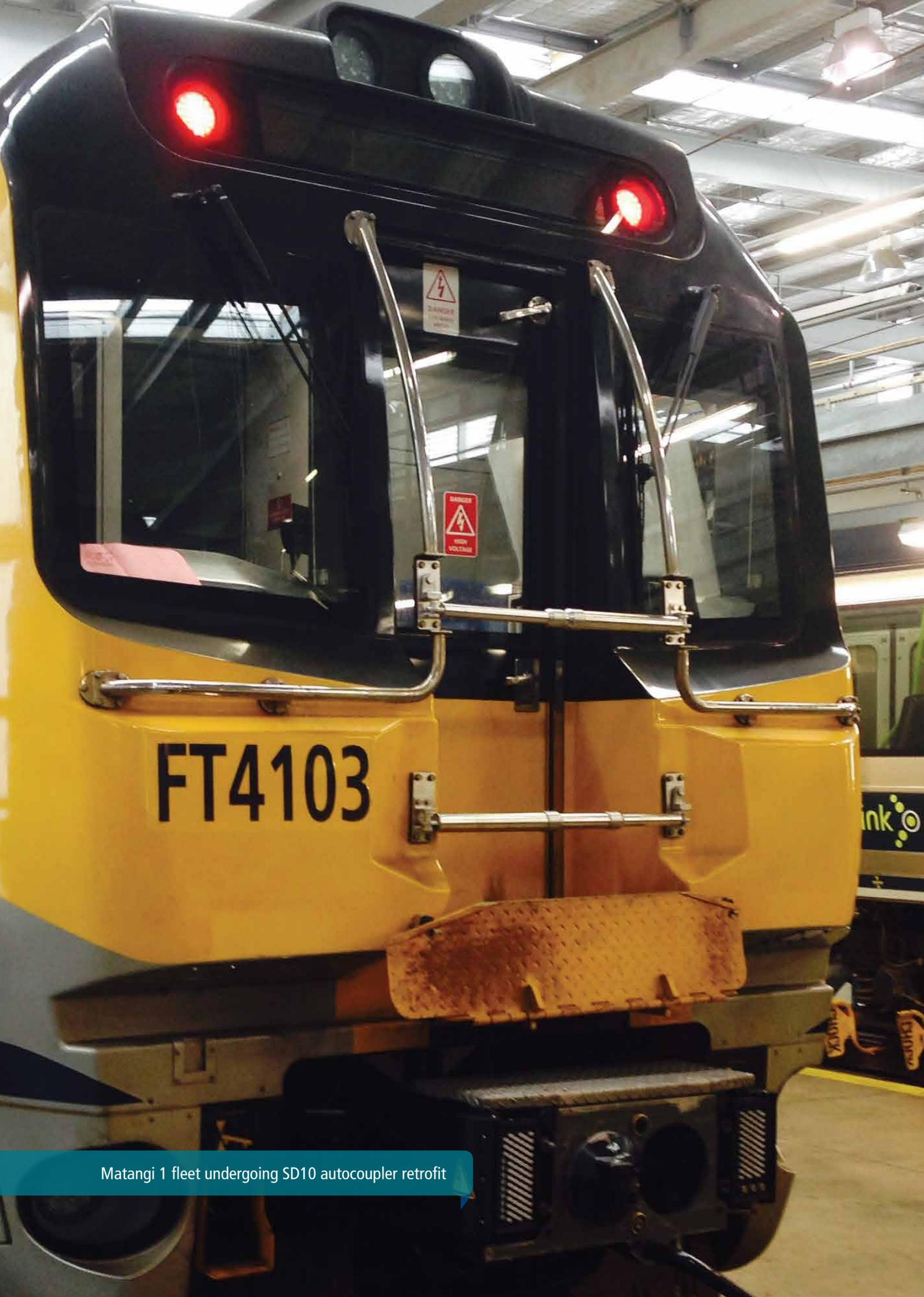
Matangi 1 fleet undergoing SD10 autocoupler retrofit
