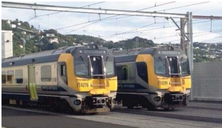
First two Matangi 1 trains fitted with auto couplers
