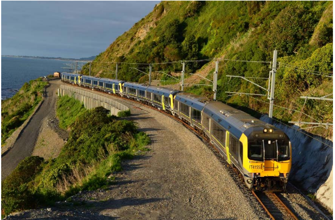
An 8-car (4 x 2-car units) Matangi train navigates the single track section at North-South Junction on the Kapiti Line. Photo courtesy of Michael Kilgour
