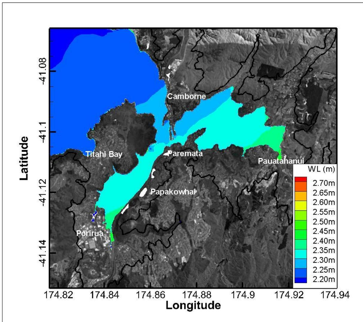
**Figure H-26: Total inundation water levels relative to WVD-53 at Porirua with 0.5 m sea-level rise.** The simulation is based on the 6 September 1994 event. White regions show areas with elevations below storm-tide sea level but not inundated in the model. The solid black line shows the extents of the land inundation grid.
