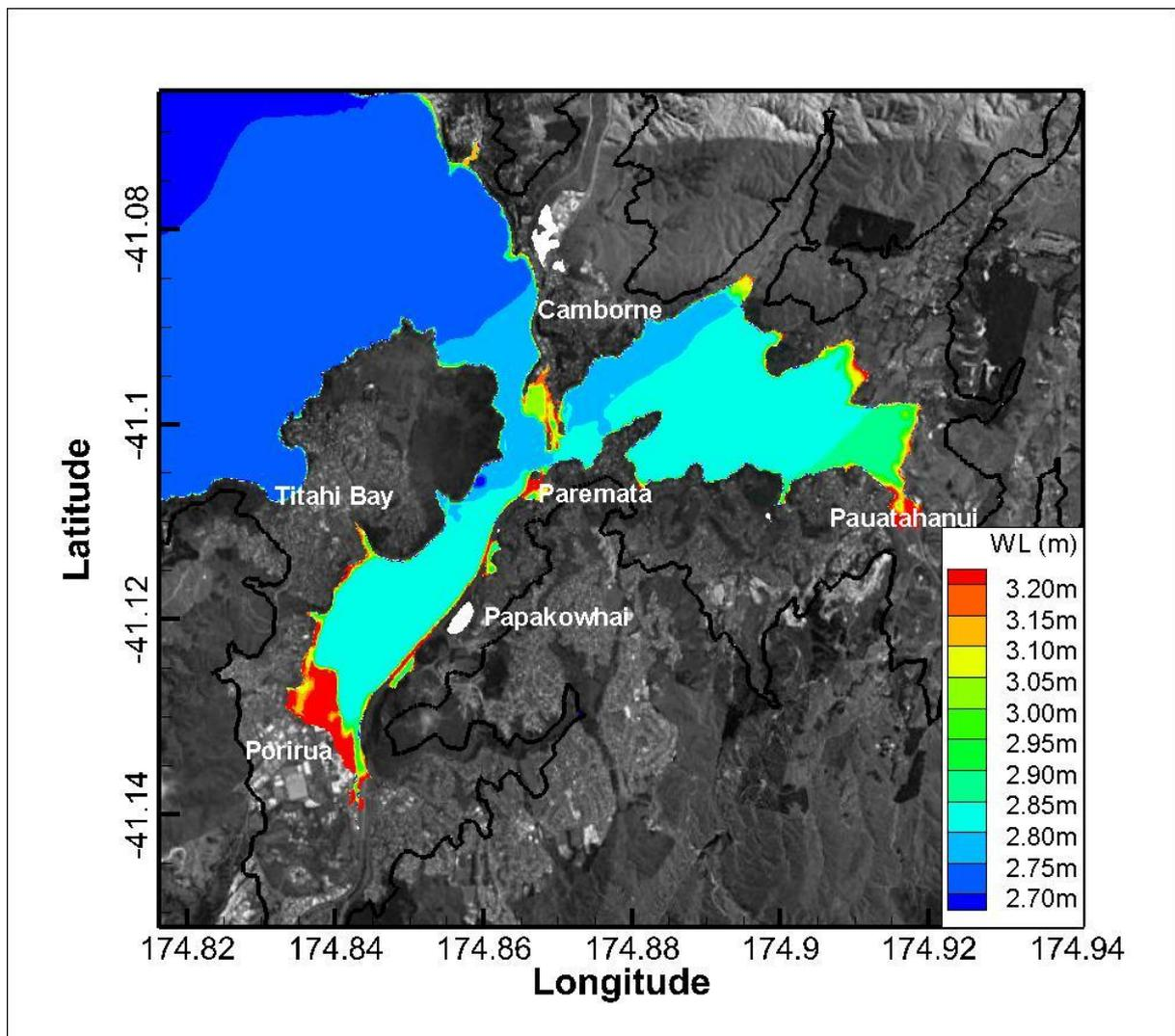
**Figure H-27: Total inundation water levels relative to WVD-53 at Porirua with 1.0 m sea-level rise.** The simulation is based on the 6 September 1994 event. White regions show areas with elevations below storm-tide sea level but not inundated in the model. The solid black line shows the extents of the land inundation grid.
