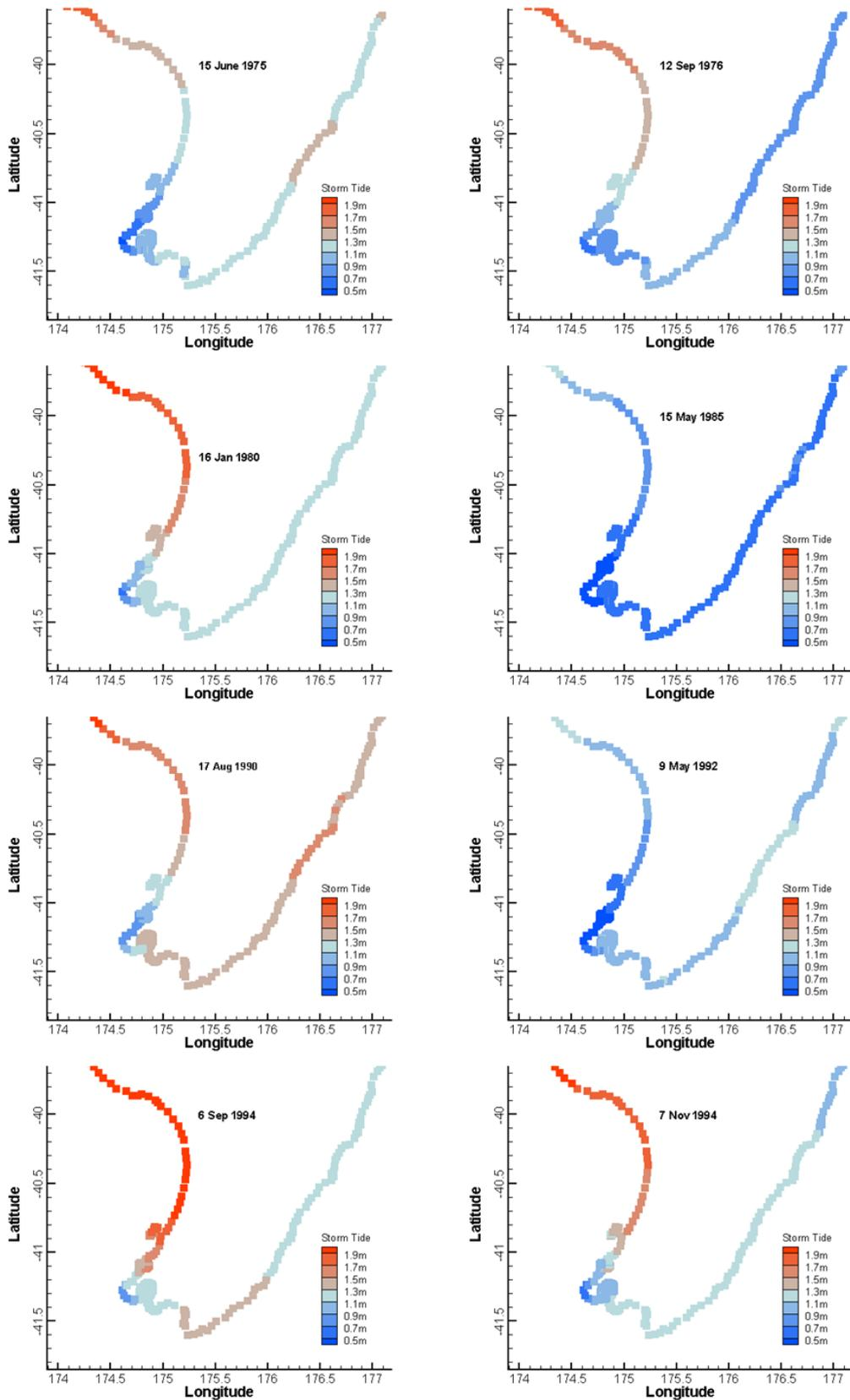
**Figure A-12: Storm-tide levels along the coast for each of the present day 1% AEP joint probability scenarios.**
