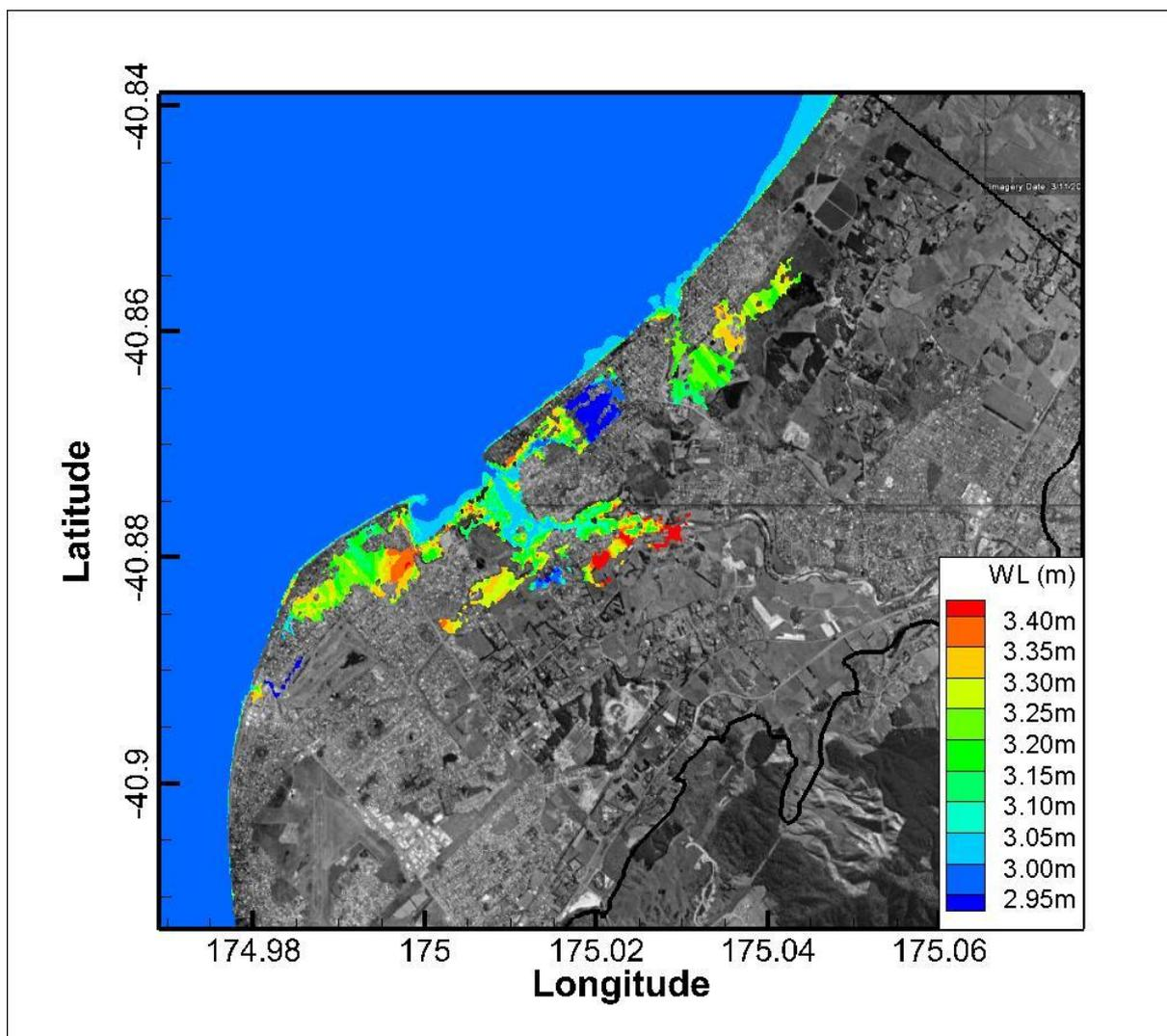
**Figure H-23: Total inundation water levels relative to WVD-53 at Waikanae with 1.0 m sea-level rise.** The simulation is based on the 6 September 1994 event. The solid black line shows the extents of the land inundation grid. White regions show areas where the topography is below storm-tide sea level, but not inundated in the modelling.
