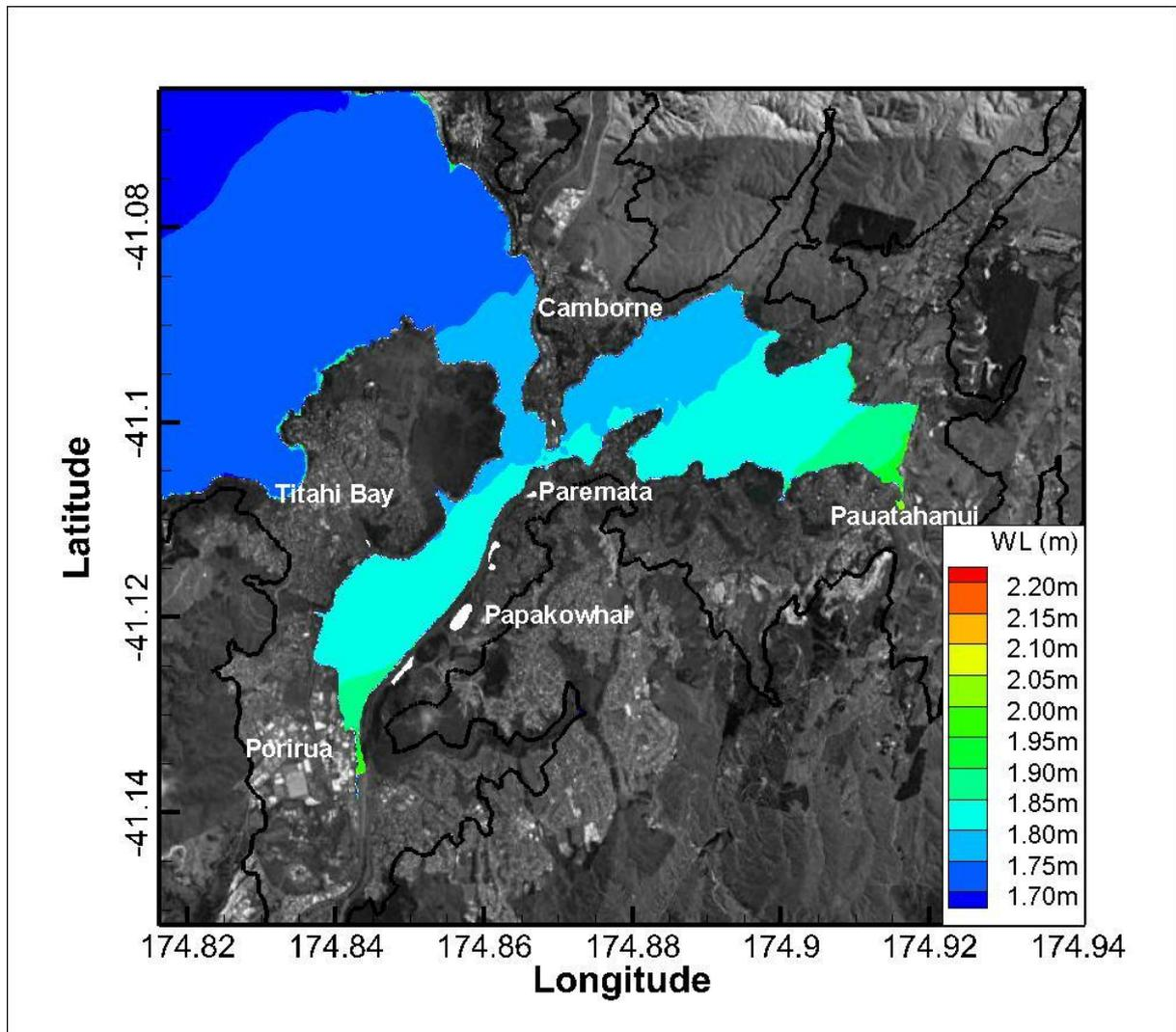
**Figure H-25: Total inundation water levels relative to WVD-53 for Porirua Harbour for the 6 September 1994 event adjusted to present day sea level and 1% joint AEP.** The colours show the maximum water level above WVD-53, overlaid on images from Google Earth. Highest astronomical tide (plus present day MLOS) is 0.952 m above WVD-53. White regions are areas with elevations lower than the sea level at the coast. The solid black line shows the extents of the land inundation grid.
