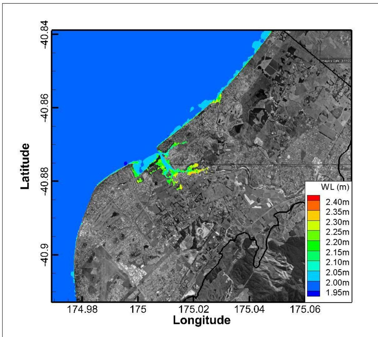
**Figure H-21: Total inundation water levels relative to WVD-53 for Waikanae for the September 1994 event adjusted to present day sea level and 1% joint AEP.** The colours show maximum water level above WVD-53, overlaid on images from Google Earth. The solid black line shows the extents of the land inundation grid. White regions show where land elevations are lower than the sea level at the coast but are not inundated in the model.
