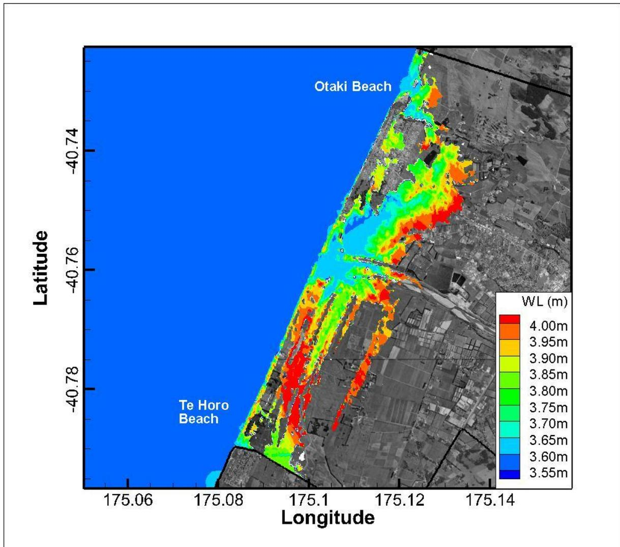
**Figure H-20: Total inundation water levels relative to WVD-53 for area near Otaki with 1.5 m sea-level rise.** The simulation is based on the 6 September 1994 event. The solid black line shows the extents of the land inundation grid. White regions indicate areas with topography below storm-tide level at the coast but not inundated in the simulation.
