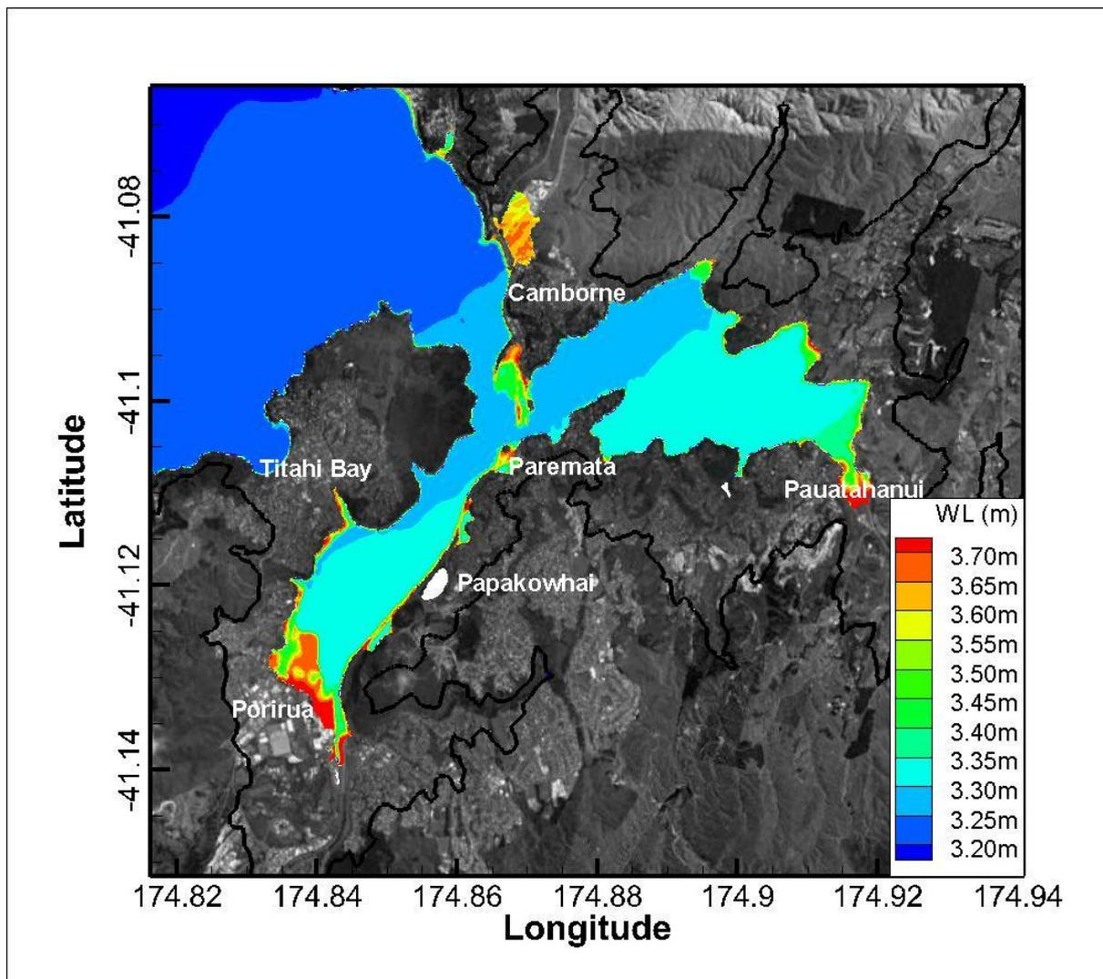
**Figure H-28: Total inundation water levels relative to WVD-53 at Porirua with 1.5 m sea-level rise.** The simulation is based on the 6 September 1994 event. White regions show areas with elevations below storm-tide sea level but not inundated in the model. The solid black line shows the extents of the land inundation grid.
