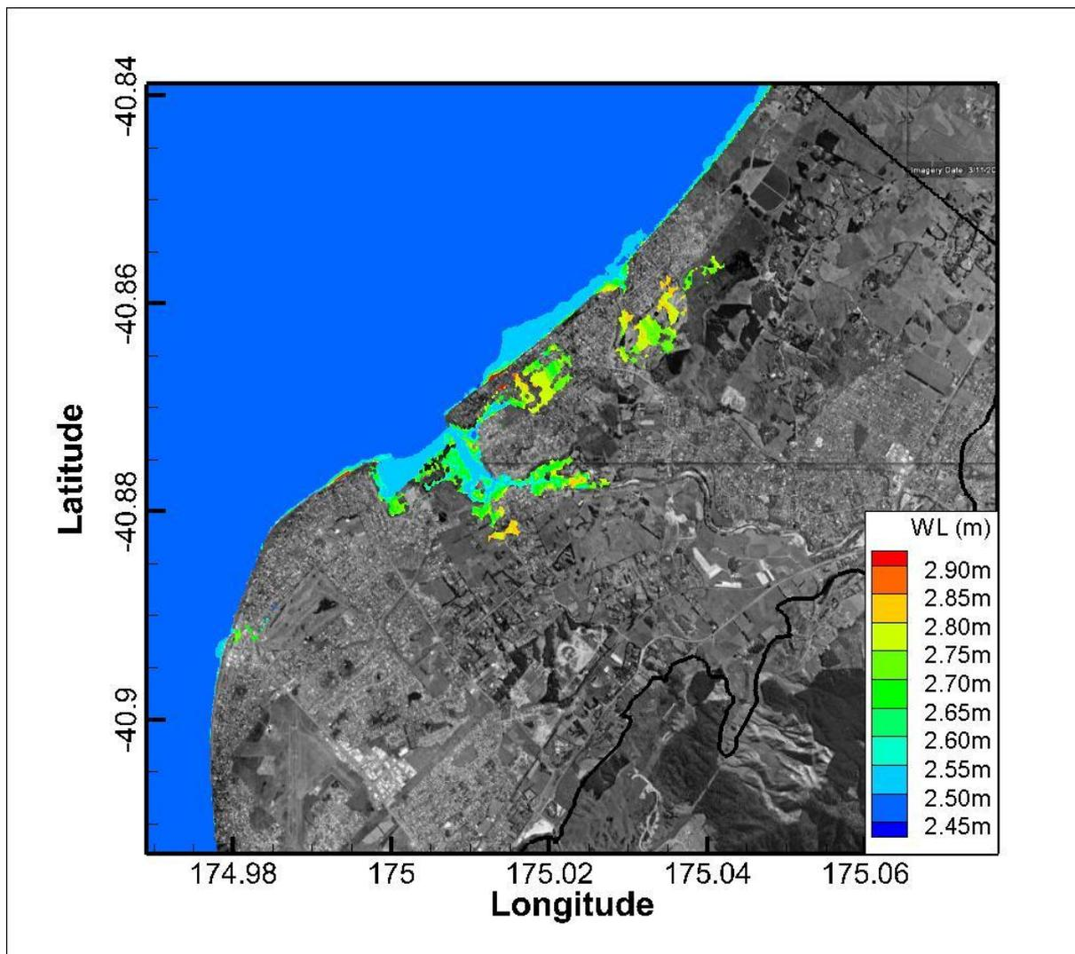
**Figure H-22: Total inundation water levels relative to WVD-53 at Waikanae with 0.5 m sea-level rise.** The simulation is based on the 6 September 1994 event. The solid black line shows the extents of the land inundation grid. White regions show areas where the topography is below storm-tide sea level, but not inundated in the modelling.
