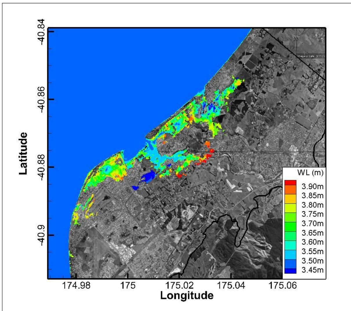
**Figure H-24: Total inundation water levels relative to WVD-53 at Waikanae with 1.5 m sea-level rise.** The simulation is based on the 6 September 1994 event. The solid black line shows the extents of the land inundation grid. White regions show areas where the topography is below storm-tide sea level, but not inundated in the modelling.
