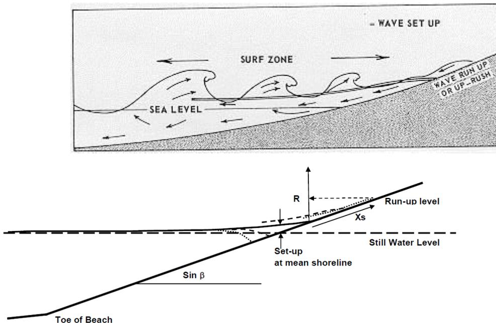
**Figure 2-2: Illustration of wave setup and runup.**
