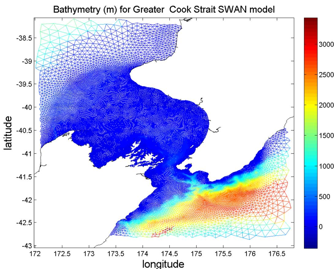
**Figure B-1: Computational mesh used for SWAN wave model simulations in the Greater Cook Strait region.**
