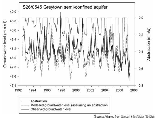
Figure 4.18: Comparison of observed groundwater levels, modelled groundwater levels (assuming no abstraction) and aquifer abstraction (extrapolated from actual metering data) for a semi-confined well (S26/0545, 18 m deep) in the Greytown groundwater management zone
