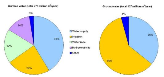
Figure 3.3: Break-down of consented surface water and groundwater allocation in the Wellington region by use type
