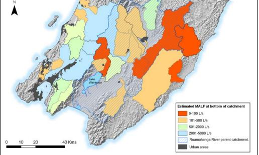
Figure 2.3: Mean annual low flow (MALF) statistics for the catchments of main rivers and streams in the Wellington region (based on estimated bottom of catchment flow statistics from Keenan 2009a and Thompson 2011a). Estimated MALF at the bottom of the Ruamahanga River parent catchment is 12,000 L/s
