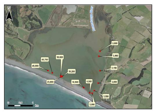
Figure 4.5: One-off conductivity values ( $\mu$ S/cm) measured at various locations in Lake Onoke on 28 August 2009, illustrating how conductivity varies spatially across the lake. The lake mouth was open at the time of this survey.
