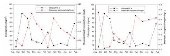
Figure 5.6: Concentrations of chlorophyll *a* alongside concentrations of dissolved reactive phosphorus (left) and nitrite-nitrate nitrogen (right), based on 11 sampling occasions in Lake Waitawa over August 2009 to July 2010
