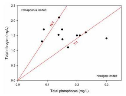
Figure 5.5: Plot of total phosphorus against total nitrogen, based on all data collected over August 2009 to July 2010. The red lines indicate thresholds for potential phosphorus limited (15:1) and nitrogen limited (7:1) conditions for phytoplankton growth. Values between the red lines are inconclusive.
