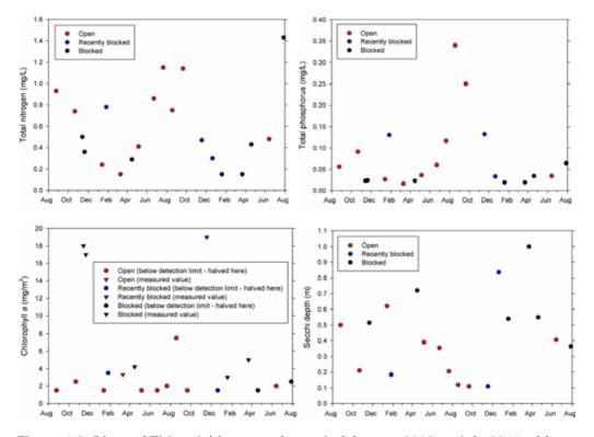
Figure 4.9: Plots of TLI variables over the period August 2009 to July 2011 with the status of the lake mouth (open, recently blocked, blocked) indicated
