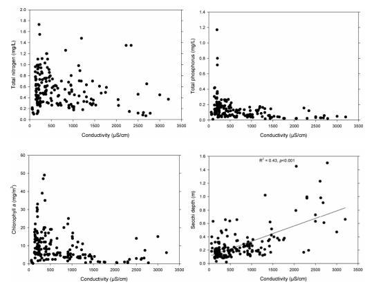
Figure 3.14: Plots of TLI variables against measurements of conductivity, based on data pooled from all four Lake Wairarapa sampling sites across the entire monitoring data record (1994–2010 where available). A linear regression line has been fitted where appropriate.
