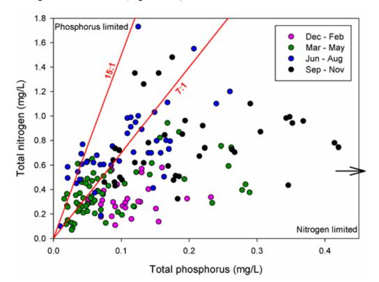
Figure 3.10: Plot of total phosphorus against total nitrogen, based on data from all sampling occasions across all four Lake Wairarapa sampling sites, coloured according to season. The red lines indicate thresholds for potential phosphorus limited (15:1) and nitrogen limited (7:1) conditions for phytoplankton growth. Values between the red lines are inconclusive. The arrow indicates the presence of three values off the scale of the graph.
