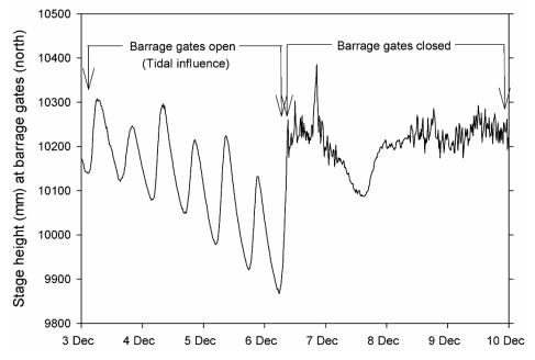
Figure 3.7: Continuous stage height measurements from the recorder located at the northern side of the barrage gates, 3 December 2009 to 10 December 2009. The status of the barrage gates (ie, open or closed) is also presented.
