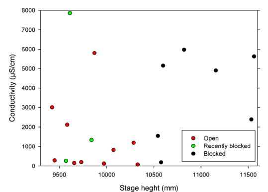
Figure 4.4: Scatter plot of lake level (stage height recorded at Lake Ferry) against measurements of conductivity. The status of the lake mouth (ie, open, recently blocked or blocked) is also shown.
