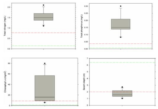
Figure 5.2: Box plots for TLI variables, based on water samples collected from Lake Waitawa over August 2008 to July 2009 (*n*=11). The horizontal dashed lines indicate national median values (taken from Verburg et al. 2010) for lakes in catchments dominated by indigenous forest (green) and pastoral (red) land cover.
