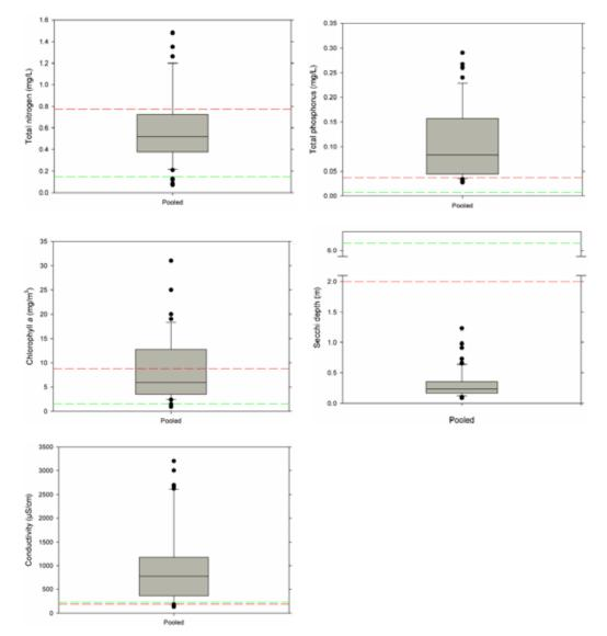
Figure 3.6: Box plots for selected water quality variables, based on data pooled for all four monitoring sites for the period 2006 to 2010. Horizontal dashed lines indicate national median values (taken from Verburg et al. 2010) for lakes in catchments dominated by indigenous forest (green) and pastoral (red) land cover.
