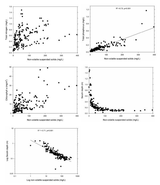
Figure 3.13: Selected variables plotted against non-volatile suspended solid (NVSS) concentrations, based on data pooled from all four sampling sites over the entire monitoring period (1994–2010). A linear regression line has been fitted where appropriate. Both actual and log transformed data are presented to demonstrate the relationship between Secchi depth and NVSS.
