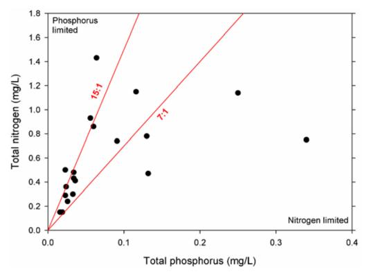
Figure 4.7: Plot of Lake Onoke total phosphorus against total nitrogen concentrations, based on data collected from Site 1 over August 2009 to July 2011. The red lines indicate thresholds for potential phosphorus limited (15:1) and nitrogen limited (7:1) conditions for phytoplankton growth. Values between the red lines are inconclusive.
