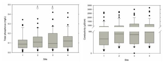
Figure 3.18: Box plots summarising differences in total phosphorus (left) and conductivity (right) concentrations between the four sampling sites, based on the entire monitoring data record (1994–2010). Arrows indicate where additional outliers are not shown. Note the *y*-axis break on the conductivity plot.
