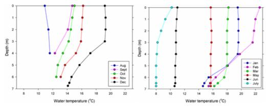
Figure 5.7: Water temperature depth profiles for Lake Waitawa, measured over August to December 2009 (left) and January to July 2010 (right)
