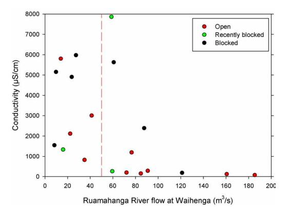
Figure 4.6: Flow recorded in the Ruamahanga River at Waihenga against conductivity measurements recorded at Site 1 in Lake Onoke. The status of the lake mouth (ie, open, recently blocked or blocked), along with the median flow of the Ruamahanga River at Waihenga (dashed vertical red line (50 m<sup>3</sup>/s), Gordon (2009)), are also shown.
