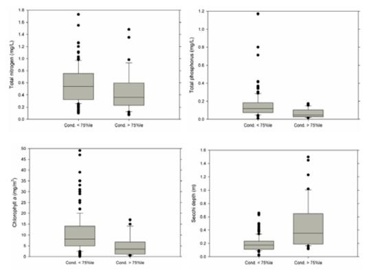
Figure 3.15: Box plots summarising the range of results for the four TLI variables for sampling occasions that coincided with conductivity values below (n=135) or above (n=45) the 75<sup>th</sup> percentile conductivity value (989 µS/cm), based on data pooled from all four Lake Wairarapa sampling sites over the entire monitoring record
