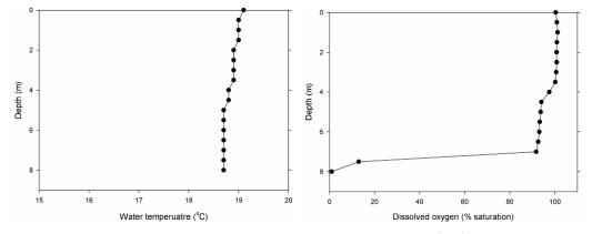
Figure 7.4: Lake Pounui depth profiles for water temperature (left) and dissolved oxygen (% saturation), based on measurements taken on 17 March 2011
