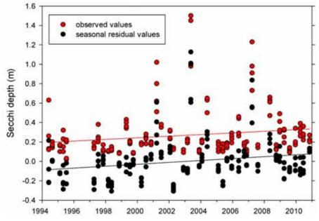
Figure 3.20: Observed Secchi depth measurements and deseasonalised residual values, based on data pooled from all four sampling sites over the period 1994 to 2010. The solid lines represent the overall trends.
