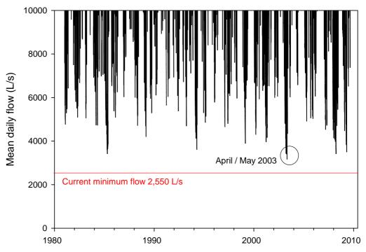
Figure 3.1: Mean daily flow for the Otaki River over 1980–2010 (only low flow portion of hydrograph shown)
