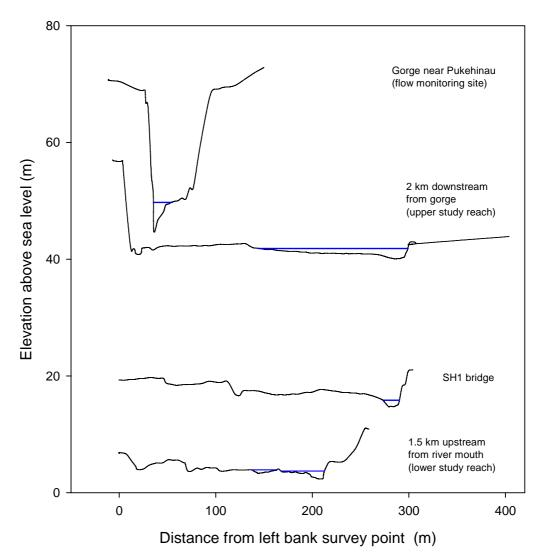
Figure 2.4: Selected Greater Wellington survey cross sections of the Otaki River channel from Pukehinau within the gorge (top section) to near the river mouth (bottom section). Elevation is metres above sea level and sections begin at the highest left bank survey point (note vertical exaggeration). Water levels on the date of survey (1 December 2005) are depicted by the blue lines.
