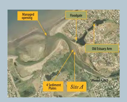
Figure 2. Sediment plate and fine scale sites, Waikanae Estuary.
