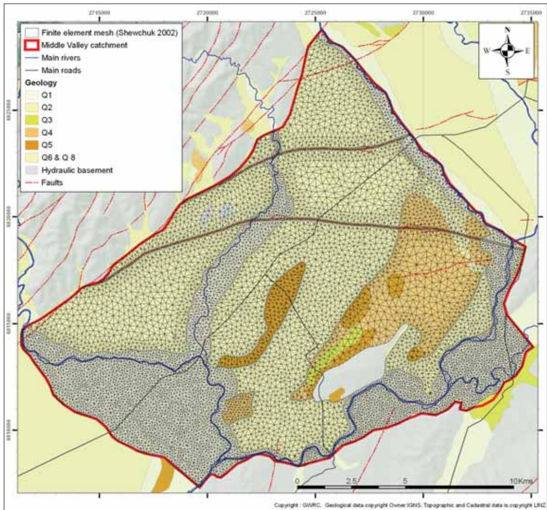
Figure 10.2: Finite element mesh for the Middle Valley catchment generated using “Triangle” (Shewchuk 2002)
