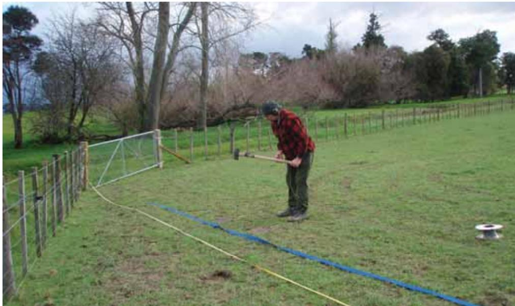
Geophysics seismic reflection survey on the Parkvale plain in July 2008. A heavy sledge hammer source with digital trigger link was selected as the seismic source. Due to the very favourable near-surface conditions and saturated ground, the hammer source provided excellent energy to over 300 ms two-way travel time.
