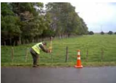
Seismic shot (sledge hammer) in action. Typically 3 shots (stacked) at each location.
